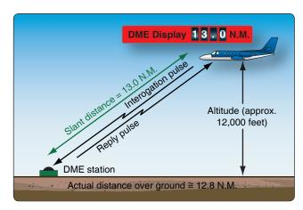
Figure 11-122. Many DME's only display the slant distance, which is the actual distance from the aircraft to the DME station. This is different than the ground distance due to the aircraft being at altitude. Some DMEs compute the ground distance for display.
