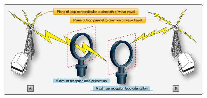
**Figure 11-93.** A loop antenna is highly direction-sensitive. A signal origin perpendicular or broadside to the loop creates a weak signal (A). A signal origin parallel or in the plain of the loop creates a strong signal (B).
