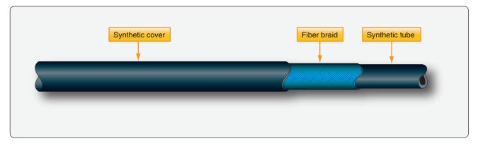
Figure 14-34. A typical flexible aircraft fuel line with braided reinforcement.
