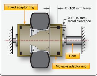
**Figure 13-149.** A ring adapter applies pressure around the entire circumference of the lower sidewall of the tire to break the bead free from the wheel rim. The diameter of the adapter must be correct for the tire and the travel limited so as to not injure the tire.
