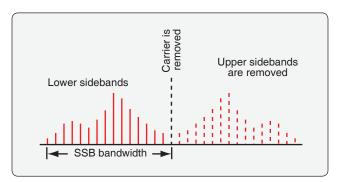
Figure 11-83. The additional frequencies above and below the carrier wave produced during modulation with the information signal are known as sidebands. Each sideband contains the unique information of the information signal and can be transmitted independent of the carrier wave and the other sideband.
