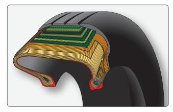
**Figure 13-129.** A radial tire has the fiber strands of the ply fabric oriented with and at 90° to the direction of rotation and the tire sidewall. This restricts flexibility directionally and the flexibility of the sidewall while it strengthens the tire to carry heavy loads.
