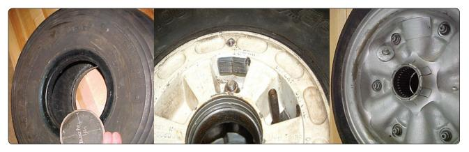
**Figure 13-159.** A tire balancing patch (left), adhesive wheel weights (center), and a bolted wheel weight (right) are all used to balance aircraft tire and wheel assemblies per the manufacturer's instructions.
