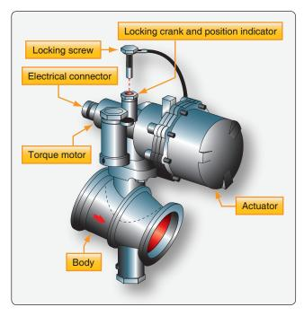
Figure 15-10. A wing anti-ice valve.
