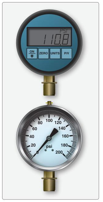
**Figure 13-133.** A calibrated bourdon tube dial-type pressure gauge or a digital pressure gauge is recommended for checking tire pressure.
