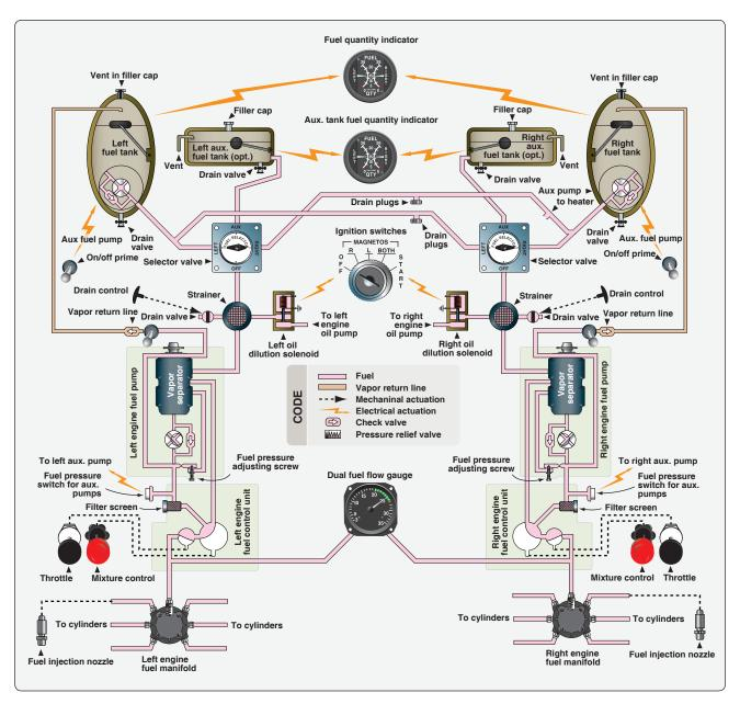
Figure 14-16. A low-wing, twin-engine, light aircraft fuel system.
