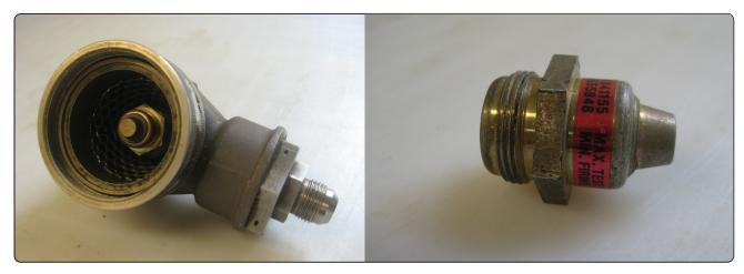
Figure 17-14. Discharge valve (left) and cartridge, or squib (right).
