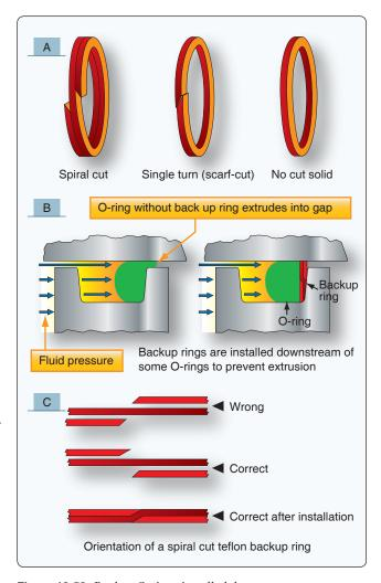
$\textbf{Figure 12-59.} \ \textit{Backup O-rings installed downstream}.$
