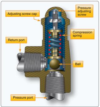
Figure 12-44. Pressure relief valve.
