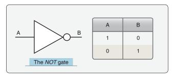
Figure 11-61. A NOT logic gate symbol and a NOT gate truth table.
