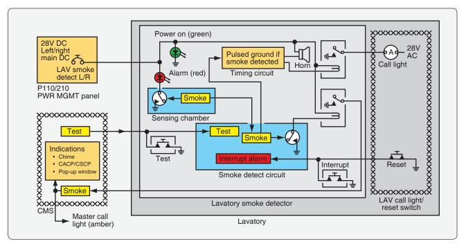
Figure 17-23. Lavatory smoke detector diagram.
