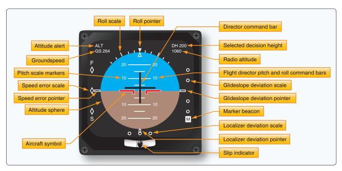
Figure 10-115. Some of the many parameters and features of an electronic attitude director indicator (EADI).
