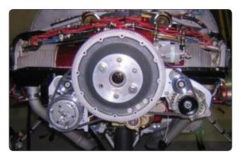
**Figure 16-81.** A typical belt drive engine driven compressor. The electromagnetic clutch pulley assembly in the front starts and stops the compressor depending on cooling demand.
