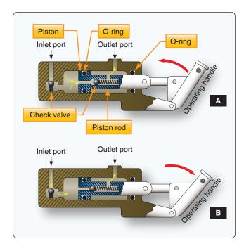
Figure 12-19. Double action hand pump.
