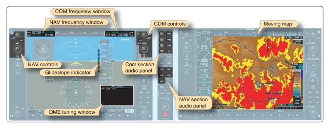
Figure 10-8. Navigation instruments.
