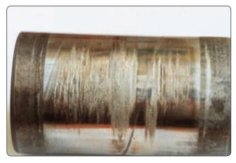
Figure 13-64. Galling is caused by rubbing of mating surfaces. The metal gets so hot it welds, and the surface metal is destroyed as the motion continues and pulls the metal apart in the direction of motion.
