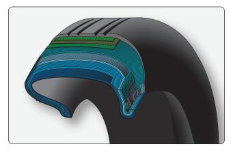
Figure 13-128. A bias ply tire has the fabric bias oriented with and across the direction of rotation and the sidewall. Since fabric can stretch on the bias, the tire is flexible, and can absorb loads. Strength is obtained by adding plies.
