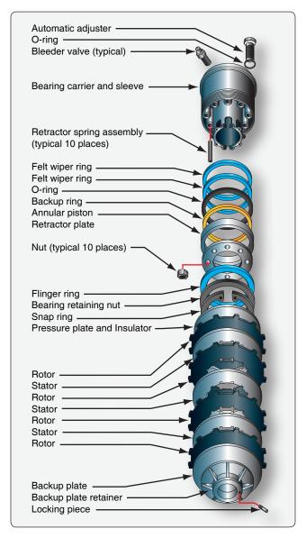
**Figure 13-84.** A multiple disc brake with bearing carrier upon which the parts of the brake are assembled including an annular cylinder and piston assembly that apply pressure evenly to a stack of rotors and stators.
