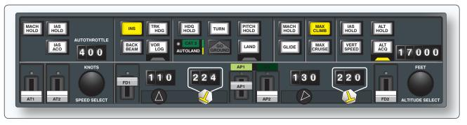
**Figure 10-112.** The AFCS control panel commands several integrated systems from a single panel including: flight directors, autopilots, autothrottles, autoland, and navigational aids. Mode selections for many features are made from this single interface.
