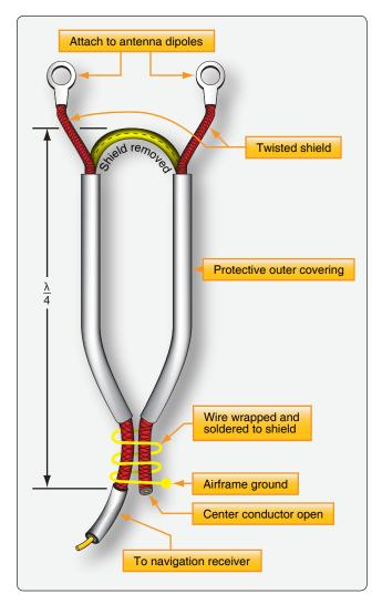
**Figure 11-163.** A balun in a dipole antenna installation provides the proper impedance for efficient power transfer.
