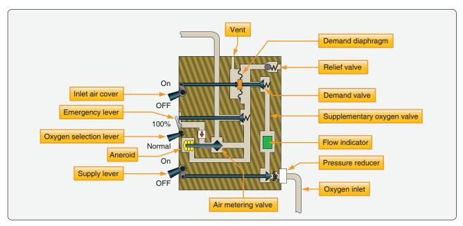
**Figure 16-21.** A diluter-demand regulator operates when low pressure caused by inhalation moves the demand diaphragm. A demand valve connected to the diaphragm opens, letting oxygen flow through the metering valve. The metering valve adjusts the mixture of cabin air and pure oxygen via a connecting link to an aneroid that responds to cabin altitude.
