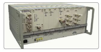
Figure 11-139. An ADS-B test unit.
