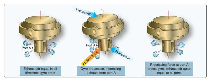
Figure 10-101. The erecting mechanism of a vacuum-driven attitude indicator.
