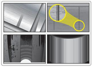
**Figure 13-67.** Brinelling is caused by excessive impact. It appears as indentations in the bearing cup raceways. Any static overload or severe impact can cause true brinelling, which leads to vibration and premature bearing failure.
