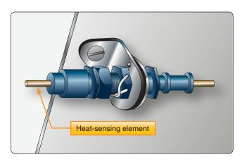
**Figure 17-26.** *Connector joint fitting attached to the structure.*
