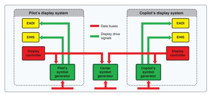
**Figure 10-118.** A simplified diagram of an EFIS system. The EADI and EHSI displays are CRT units in earlier systems. Modern systems use digital displays, sometimes with only one multifunctional display unit replacing the two shown. Independent digital processors can also be located in a single unit to replace the three separate symbol generators.
