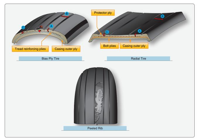
**Figure 13-139.** Remove an aircraft tire from service when the depth of a cut exposes the casing outer plies of a bias ply tire or the outer belt layer of a radial tire (A); a tread rib has been severed across the entire width (B); or, when undercutting occurs at the base of any cut (C). These conditions may lead to a peeled rib.
