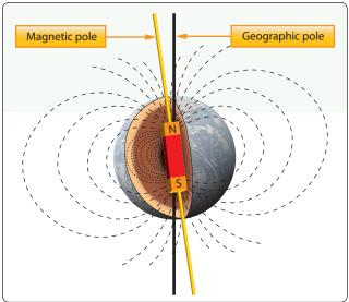
Figure 10-78. The earth and its magnetic field.
