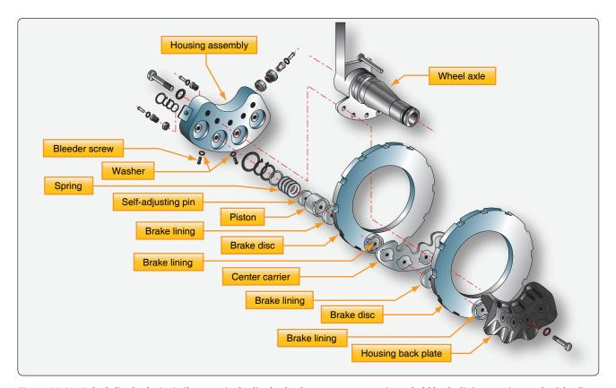
Figure 13-83. A dual-disc brake is similar to a single-disc brake. It uses a center carrier to hold brake linings against each of the discs.
