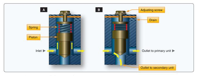
Figure 12-39. A pressure-controlled sequence valve.
