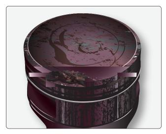
**Figure 14-7.** Preignition can cause detonation and damage to the engine.
