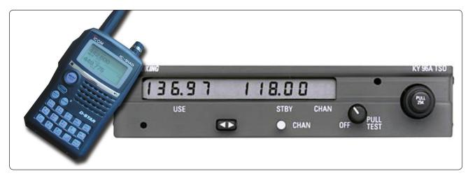
Figure 11-86. VHF aircraft communication transceivers.
