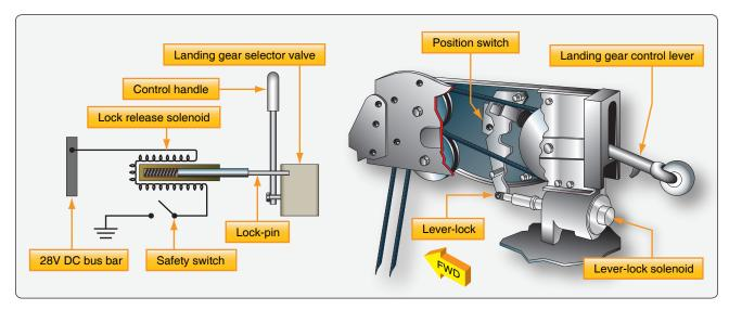
**Figure 13-40.** A landing gear safety circuit with solenoid that locks the control handle and selector valve from being able to move into the gear up position when the aircraft is on the ground. The safety switch, or squat switch, is located on the aircraft landing gear.
