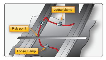
Figure 17-27. Rubbing interference.
