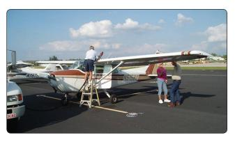
Figure 14-105. Over-the-wing refueling a Cessna.
