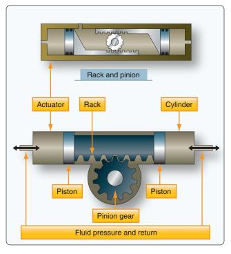
Figure 12-54. Rack and pinion gear.
