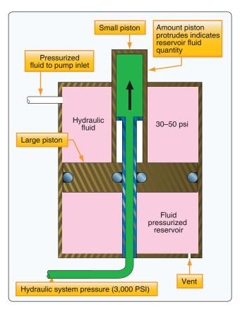
**Figure 12-13.** Operating principle behind a fluid-pressurized hydraulic reservoir.
