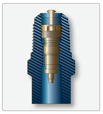
**Figure 16-84.** *Cross-section of an R12 refrigerant service valve.*
