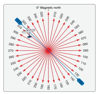
Figure 11-97. A VOR transmitter produces signals for 360° radials that an airborne receiver uses to indicate the aircraft's location in relation to the VOR station regardless of the aircraft's direction of flight. The aircraft shown is on the 315° radial even though it does not have a heading of 315°.
