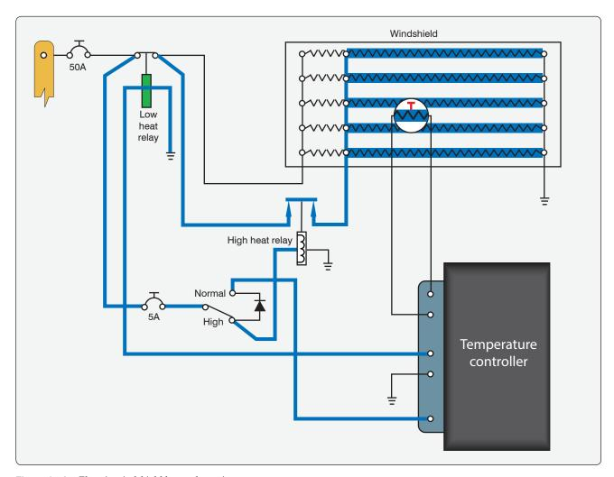
**Figure 15-45.** *Electric windshield heat schematic.*
