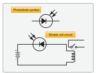
**Figure 11-38.** The symbol for a photodiode and a photodiode in a simple coil circuit.
