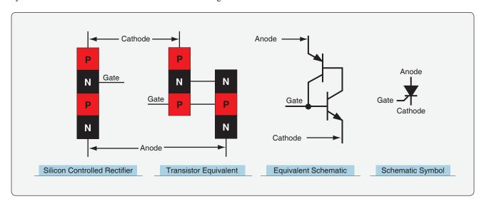
**Figure 11-29.** A silicon controlled rectifier (SCR) allows current to pass in one direction when the gate receives a positive pulse to latch the device in the on position. Current ceases to flow when it drops below holding current, such as when AC current reverses cycle.
