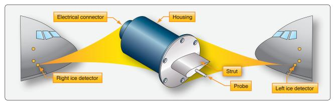
**Figure 15-4.** An ice detector alerts the flight crew of icing conditions and, on some aircraft, automatically activates ice protection systems. One or more detectors are located on the forward fuselage.
