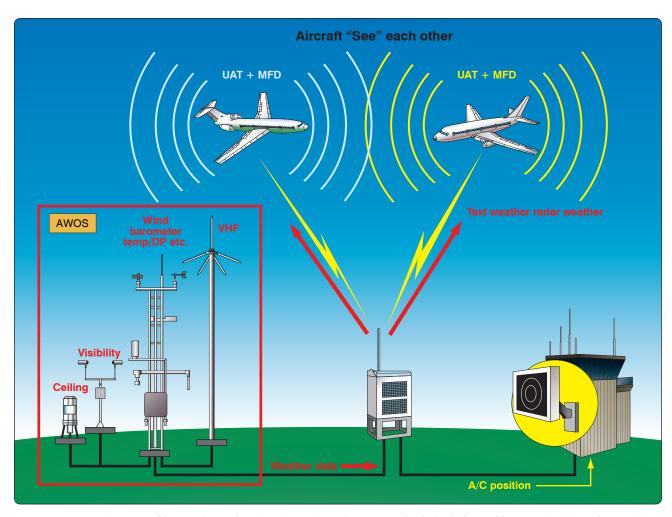
**Figure 11-138.** ADS-B IN enables weather and traffic information to be sent into the flight deck. In addition to AWOS weather, NWS can also be transmitted.
