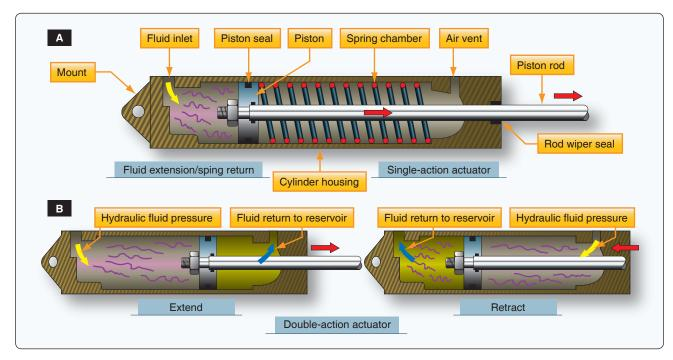
Figure 12-52. Linear actuator.
