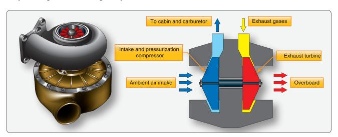
Figure 16-44. A turbocharger used for pressurizing cabin air and engine intake air on a reciprocating engine aircraft.
