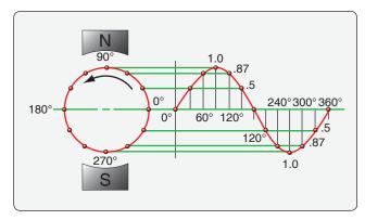
**Figure 11-55.** Voltage over time of sine waveform electricity created when a conductor is rotated through a uniform magnetic field, such as in a generator.
