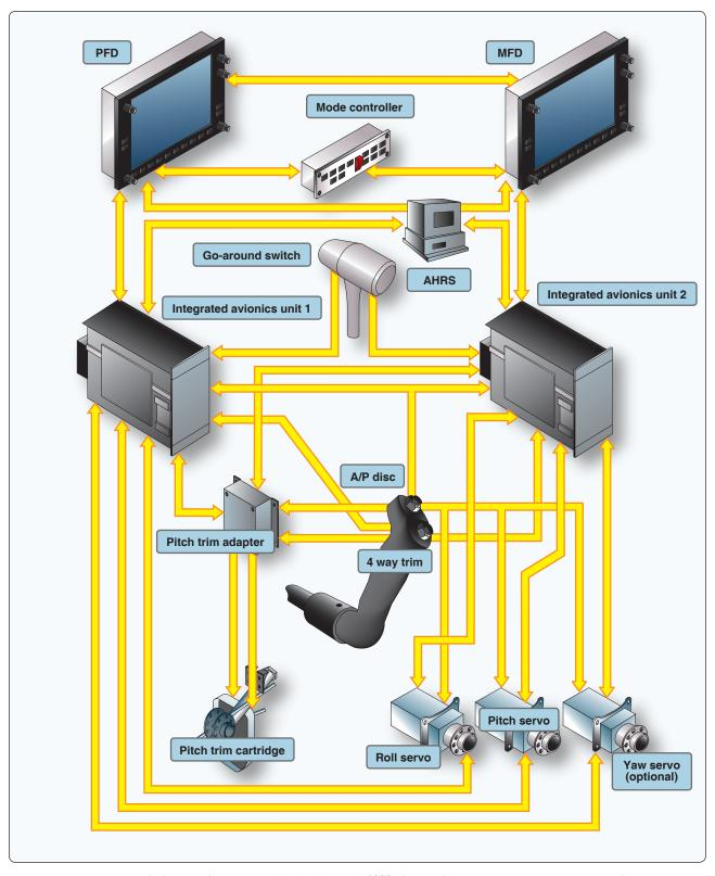
$\textbf{Figure 10-113.} \ \textit{Automatic flight control system (AFCS) of a Garmin G1000 glass cockpit instrument system for a general aviation aircraft.$
