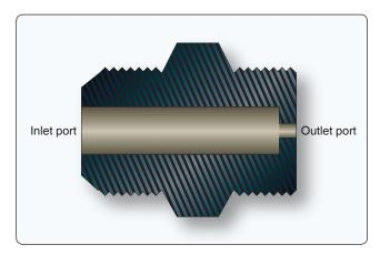
Figure 12-74. Pneumatic orifice valve.
