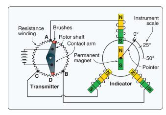
**Figure 10-47.** A schematic of a DC selsyn synchro remote indicating system.
