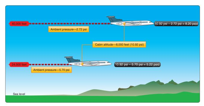
**Figure 16-41.** Differential pressure (psid) is calculated by subtracting the ambient air pressure from the cabin air pressure.
