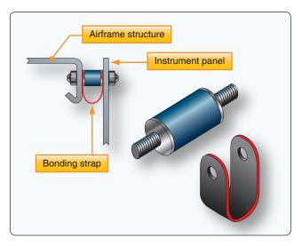
Figure 10-133. *Instrument panel shock mounts.*
