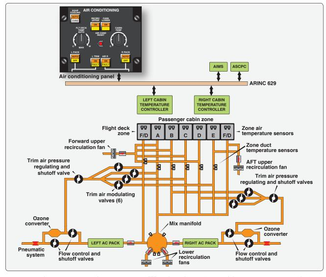
**Figure 16-71.** The temperature control system of a Boeing 777 combines the use of zone and duct temperature sensors with trim air modulating valves for each zone. Redundant digital left and right cabin temperature controllers process temperature input signals from the sensors and temperature selectors on the cockpit panel and throughout the aircraft to modulate the valves.
