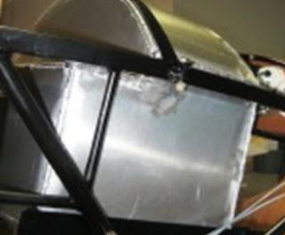
**Figure 14-90.** A rigid removable fuel tank with welded seams is repaired by welding.
