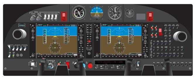
**Figure 11-70.** A modern glass cockpit on a general aviation aircraft. Digital data displays replace many older instruments and indicators of the past.
