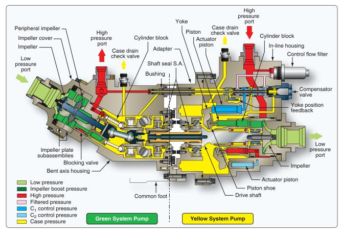
Figure 12-57. Power transfer unit.
