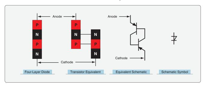
**Figure 11-28.** A four-layer semiconductor diode behaves like two transistors. When breakover voltage is reached, the device conducts current until the voltage is removed.
