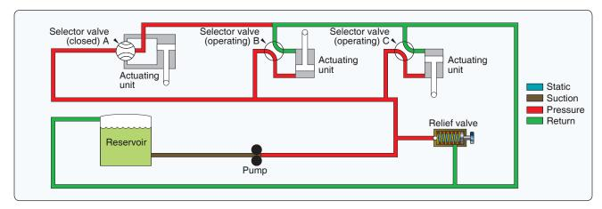
Figure 12-4. A basic closed-center hydraulic system with a variable displacement pump.
