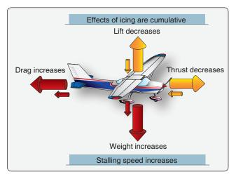
Figure 15-2. Effects of structural icing.
