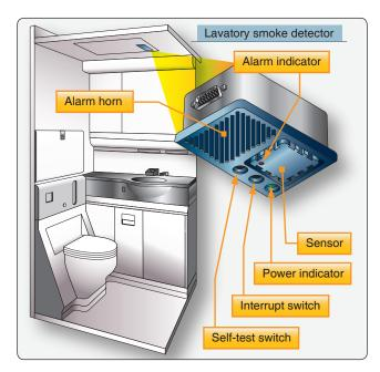
Figure 17-22. Lavatory smoke detector diagram.
