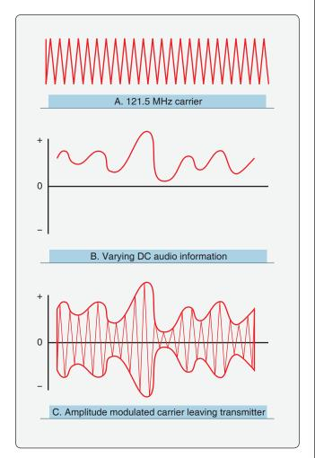
Figure 11-79. A DC audio signal modifies the 121.5 MHz carrier wave as shown in C. The amplitude of the carrier wave (A) is changed in relation to modifier (B). This is known as amplitude modulation (AM).
