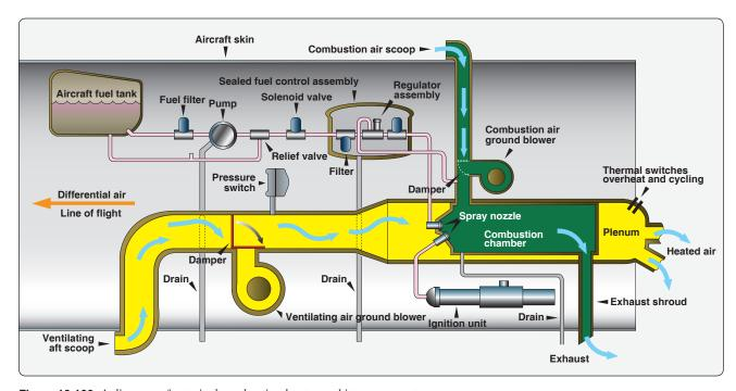
$\textbf{Figure 16-100.} \ A \ diagram \ of \ a \ typical \ combustion \ heater \ and \ its \ components.$
