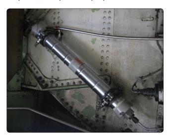
Figure 12-50. Cylindrical accumulator.
