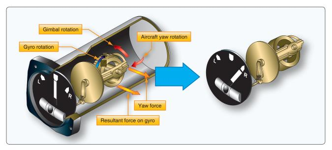
Figure 10-106. The turn-and-slip indicator's gyro reaction to the turning force in a right hand turn. The yaw force results in a force on the gyro 90° around the rotor in the direction it is turning due to precession. This causes the top of the rotor to tilt to the left. Through connecting linkage, the pointer tilts to the right.
