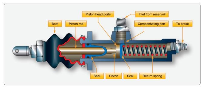
Figure 13-94. A Goodyear brake master cylinder from an independent braking system with a remote reservoir.
