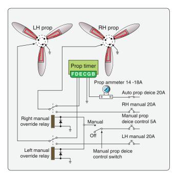
**Figure 15-36.** *Propeller electrical deice system schematic.*
