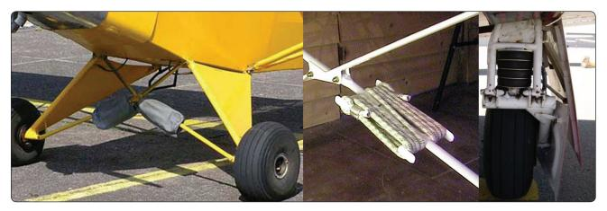
**Figure 13-15.** Piper Cub bungee cord landing gear transfer landing loads to the airframe (left and center). Rubber, donut-type shock transfer is used on some Mooney aircraft (right).
