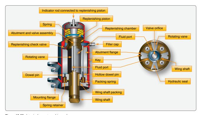
$\textbf{Figure 13-55.} \ A \ typical \ vane-type \ shimmy \ damper.$
