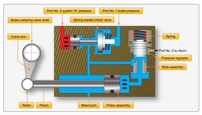
Figure 13-100. The power brake system on a Boeing 737.
