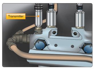
**Figure 10-18.** A hydraulic pressure transmitter senses and converts pressure into an electrical output for indication by the cockpit gauge or for use by a computer that analyzes and displays the pressure in the cockpit when requested or required.
