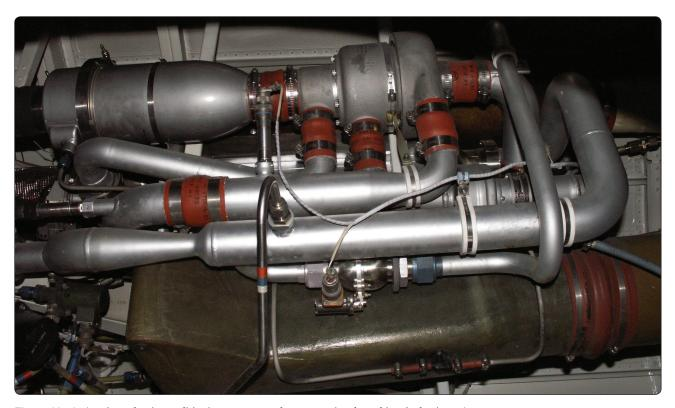
**Figure 16-50.** An air cycle air conditioning system used to pressurize the cabin of a business jet.
