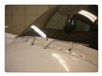
Figure 15-46. Chemical deicing spray tubes.
