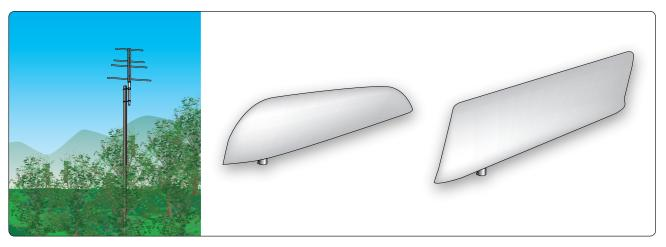
**Figure 11-117.** An outer marker transmitter antenna 4–7 miles from the approach runway transmits a 75 MHz signal straight up (left). Aircraft mounted marker beacon receiver antennas are shown (center and right).
