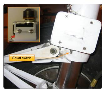
Figure 13-39. Typical landing gear squat switches.
