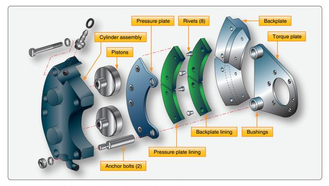
**Figure 13-82.** An exploded view of a dual-piston Cleveland brake assembly.
