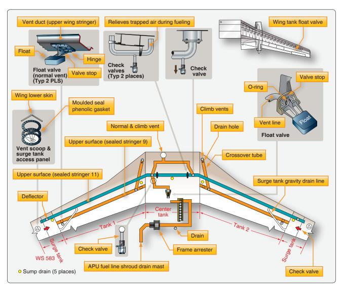
**Figure 14-20.** A fuel vent system with associated float and check valves that stop fuel and keep the tanks vented regardless of the aircraft attitude.
