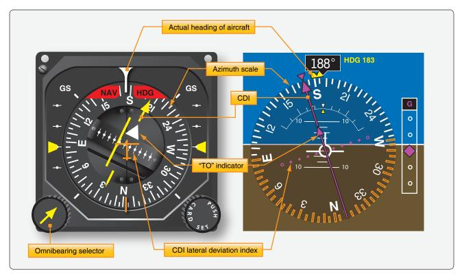
Figure 11-102. A mechanical HSI (left) and an electronic HSI (right) both display VOR information.
