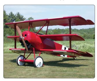
**Figure 13-14.** Rigid steel landing gear is used on many early aircraft.
