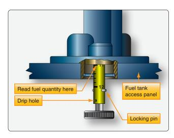
Figure 14-75. A fuel drip stick is lowered from the fuel tank bottom until fuel drips out the hole at the bottom. By reading the calibrated scale and adding readings from all tank drip sticks, a chart can be consulted to arrive at the total fuel quantity on the aircraft by weight or by volume.
