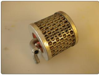
Figure 15-29. Air filter for vacuum system.
