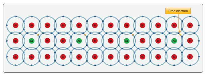
**Figure 11-17.** Silicon atoms doped with arsenic form a lattice work of covalent bonds. Free electrons exist in the material from the arsenic atom's 5th valence electron. These are the electrons that flow when the semiconductor material, known as N-type or donor material, is conducting.
