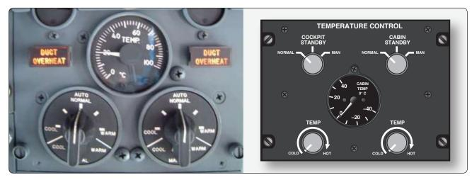
**Figure 16-70.** Typical temperature selectors on a transport category aircraft temperature control panel in the cockpit (left) and a business jet (right). On large aircraft, temperature selectors may be located on control panels located in a particular cabin air distribution zone.
