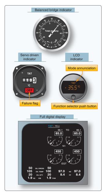
Figure 10-76. Different cockpit TAT displays.
