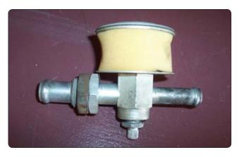
Figure 10-89. A vacuum regulator, also known as a suction relief valve, includes a foam filter. To relieve vacuum, outside air of a higher pressure must be drawn into the system. This air must be clean to prevent damage to the pump.
