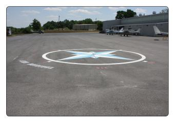
**Figure 10-140.** *The compass rose on this airport ramp can be used to swing an aircraft magnetic compass.*
