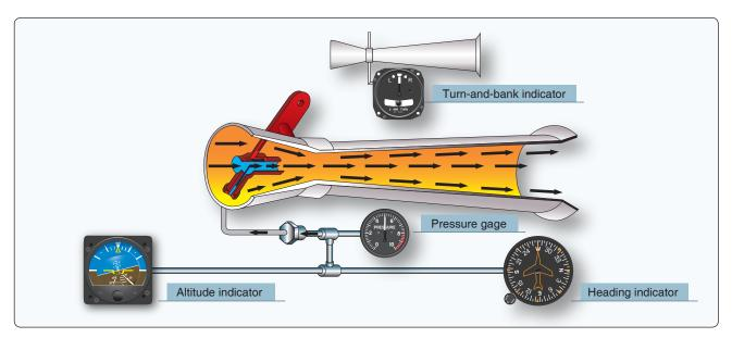
**Figure 10-87.** *Simple venturi tube systems for powering gyroscopic instruments.*
