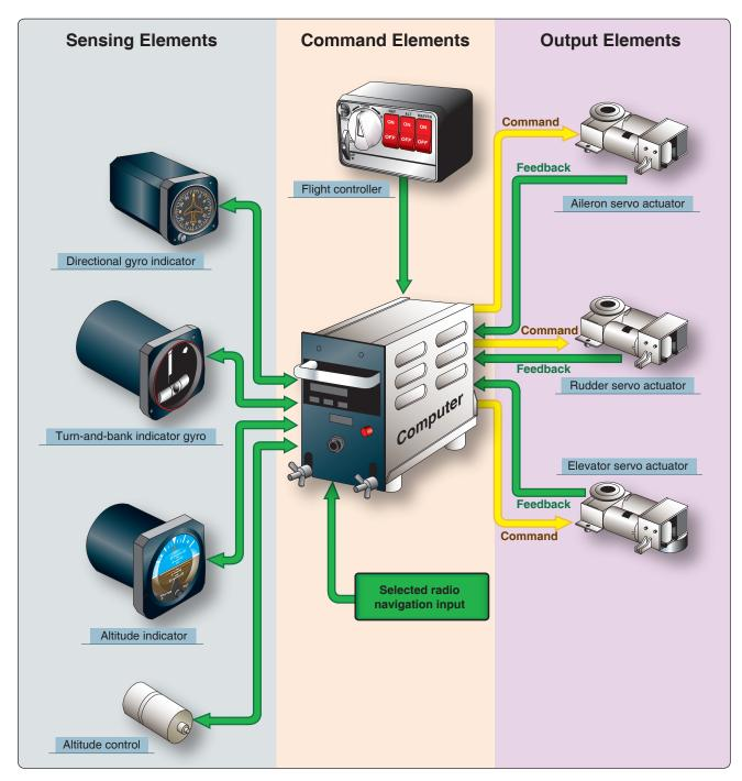
Figure 10-108. Typical analog autopilot system components.
