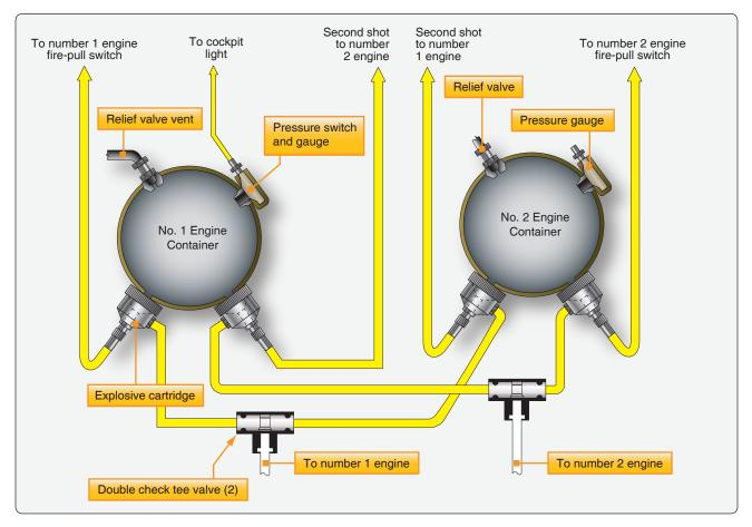
Figure 17-13. Diagram of fire extinguisher containers (HRD bottles).
