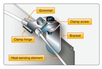
Figure 17-28. Inspection of fire detector loop clamp.
