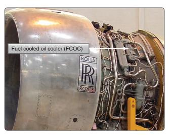
**Figure 14-23.** *Jet transport aircraft fly at high altitudes where temperatures can reach* –50 °F. *Most have fuel heaters somewhere in the fuel system to help prevent fuel icing. This fuel-cooled oil cooler on an RB211 turbofan engine simultaneously heats the fuel while cooling the oil.*
