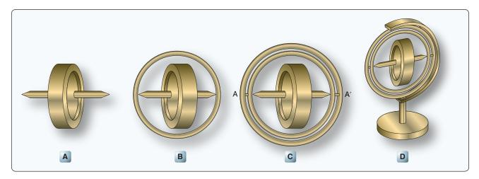
Figure 10-93. Gyroscopes.
