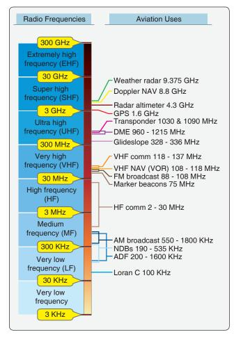
**Figure 11-75.** There is a wide range of radio frequencies. Only the very low frequencies and the extremely high frequencies are not used in aviation.
