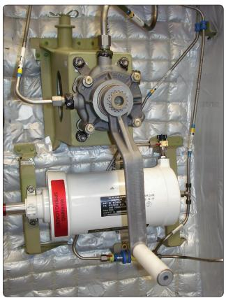
Figure 12-20. Rotary hand pump.
