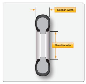
**Figure 13-125.** Type III aircraft tires are identified via a two-number system with a (-) separating the numbers. The first number is the tire section width in inches. The second number is the rim diameter in inches. For example: 6.00-6 is a Cessna 172 tire that is 6.00 inches wide and fits on a rim that has a diameter of 6 inches.
