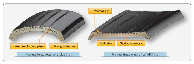
Figure 13-135. Normal tire wear.
