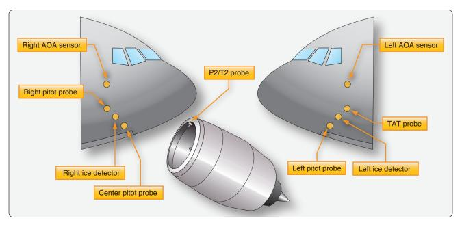
Figure 15-14. Probes with thermal electric anti-icing on one commercial airliner.
