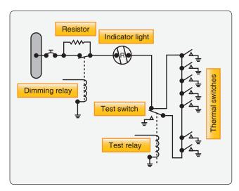
Figure 17-1. Thermal switch fire circuit.
