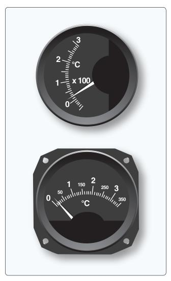
**Figure 10-73.** *Typical thermocouple temperature indicators.*
