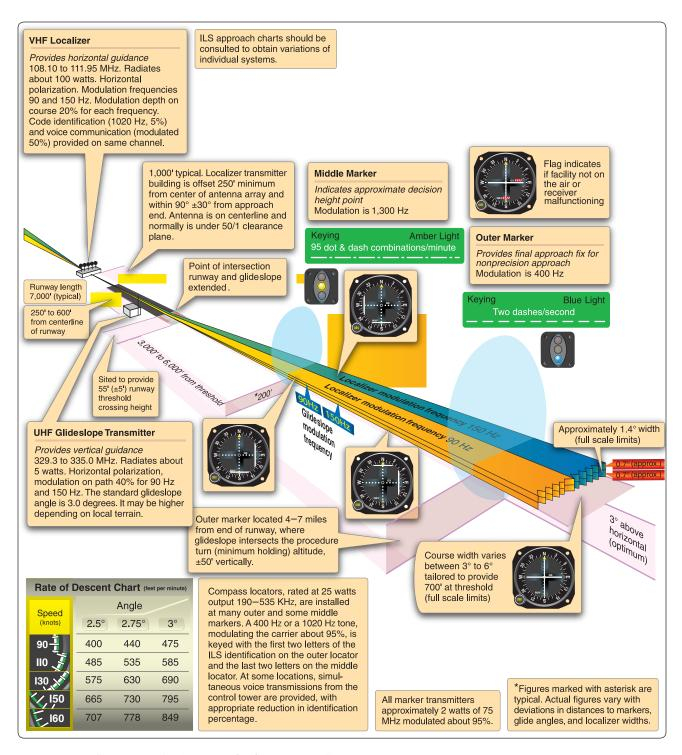
Figure 11-110. Components of an instrument landing system (ILS).
