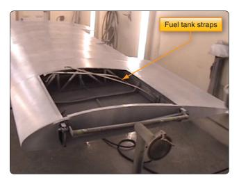
**Figure 14-28.** A fuel tank bay in the root of a light aircraft wing on a stand in a paint booth. Padded straps hold the fuel tank securely in the structure.
