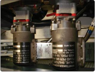
Figure 12-48. Shutoff valves.
