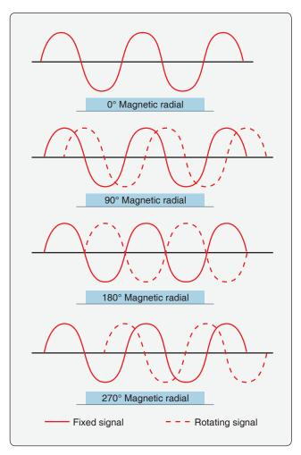
**Figure 11-98.** The phase relationship of the two broadcast VOR signals.
