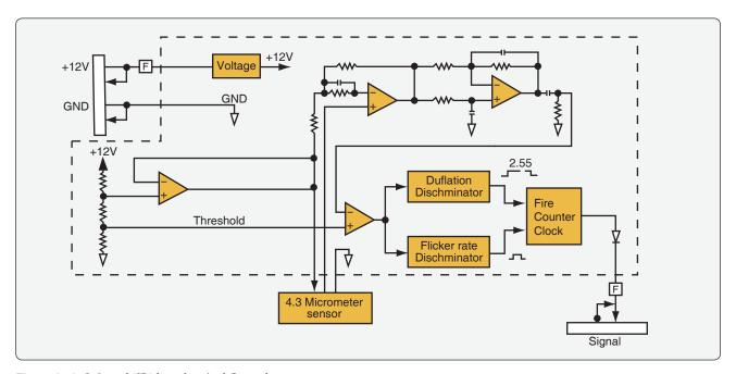
**Figure 17-9.** *Infrared (IR) based optical flame detector.*
