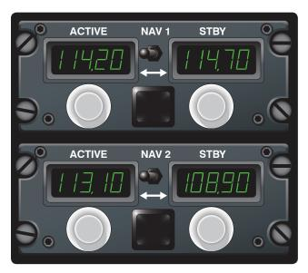
Figure 11-100. An airliner VOR control head with two independent NAV receivers each with an active and standby tuning circuit controlled by a toggle switch.
