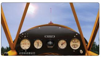
**Figure 14-66.** The fuel quantity indicator on this Piper Cub is a float attached to a rod that protrudes through the fuel cap.
