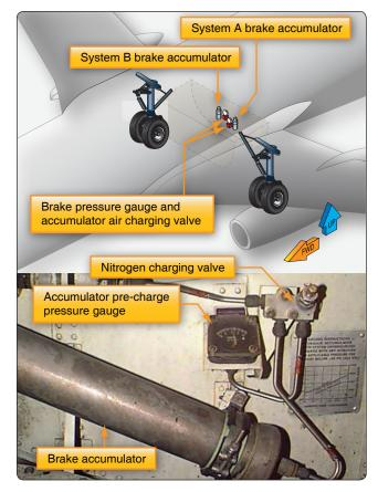
Figure 13-101. Emergency brake hydraulic fluid accumulators are precharged with nitrogen to deliver brake fluid to the brakes in the event normal and alternate hydraulic sources fail.
