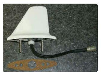
Figure 11-121. A typical aircraft-mounted DME antenna.
