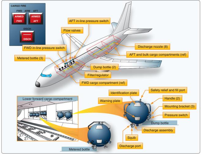
**Figure 17-21.** *Cargo and baggage compartment extinguishing system.*
