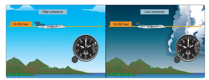
**Figure 10-35.** Above 18,000 feet MSL, all aircraft are required to set 29.92 as the reference pressure in the Kollsman window. The altimeter then reads pressure altitude. Depending on the atmospheric pressure that day, the true or actual altitude of the aircraft may be above or below what is indicated (pressure altitude).
