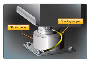
**Figure 11-159.** A bonding jumper is used to ground an equipment rack and avionics chassis around the non-conductive shock mount material.
