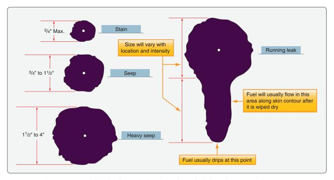
Figure 14-89. The surface area of collected fuel from a leak is used to classify the leak into the categories shown.
