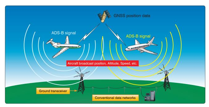
**Figure 11-136.** ADS-B OUT uses satellites to identify the position aircraft. This position is then broadcast to other aircraft and to ground stations along with other flight status information.
