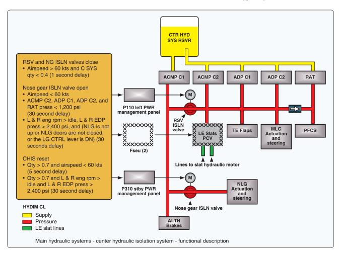
Figure 12-69. Center hydraulic isolation system.
