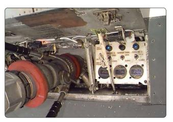
**Figure 14-21.** A central pressure refueling station on a transport category aircraft allows all fuel tanks to be filled from one position.
