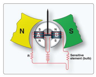
Figure 10-70. A ratiometer temperature measuring indicator has two coils. As the sensor bulb resistance varies with temperature, different amounts of current flow through the coils. This produces varying magnetic fields. These fields interact with the magnetic field of a large permanent magnet, resulting in an indication of temperature.
