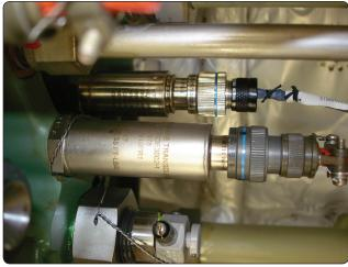
Figure 12-11. Temperature and quantity sensors.
