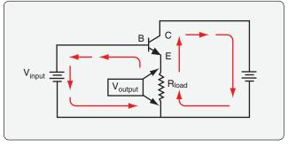
**Figure 11-48.** A basic common-collector amplifier circuit. Both the input and output circuits share a path through the load and the emitter. This causes a direct relationship of the output current to the input current.
