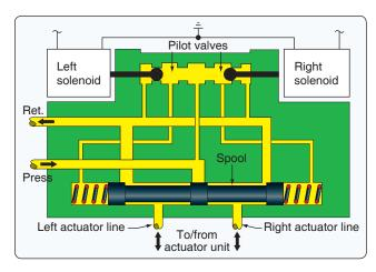
Figure 12-36. Servo control valve solenoids not energized.
