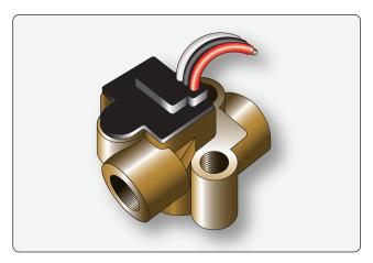
**Figure 14-81.** A turbine flow transducer in this fuel flow sensor produces a current pulse signal from an opto-electronic pickup with a preamplifier.
