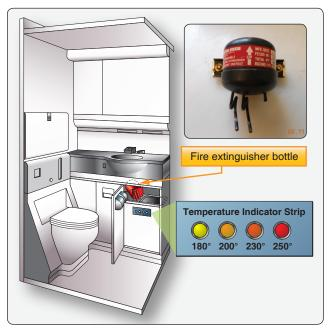
Figure 17-24. Lavatory fire extinguishing bottle.
