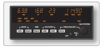
**Figure 11-124.** *RNAV unit from a general aviation aircraft.*
