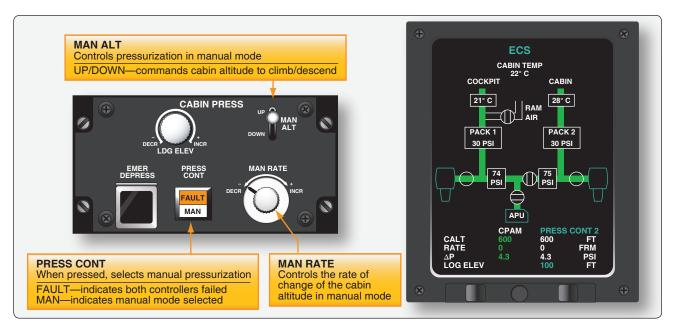
**Figure 16-58.** The pressurization panel and environmental control system page on a Bombardier CRJ200 50 passenger jet have no gauges. Traditional pressurization data is presented in digital format at the bottom of the page.
