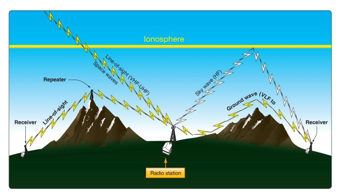
**Figure 11-78.** *Radio waves behave differently in the atmosphere depending in their frequency.*
