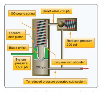
**Figure 12-46.** *Operating mechanism of a pressure reducing valve.*
