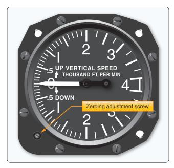
Figure 10-38. A typical vertical speed indicator.
