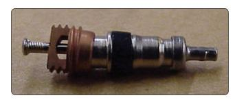
**Figure 13-148.** The tire valve core should be removed after the tire is completely deflated and before the tire and wheel assembly is removed from the aircraft.
