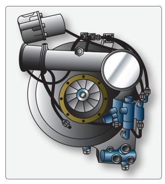
Figure 16-47. A centrifugal cabin supercharger.
