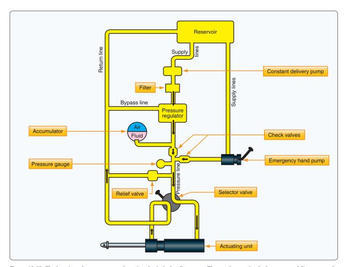
**Figure 12-45.** The location of a pressure regulator in a basic hydraulic system. The regulator unloads the constant delivery pump by bypassing fluid to the return line when the predetermined system pressure is reached.
