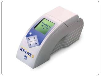
**Figure 14-99.** A capture solution is put into a 1 liter sample of fuel and shaken. The solution is then put into the analyzer shown to determine the level of microorganisms in the fuel.
