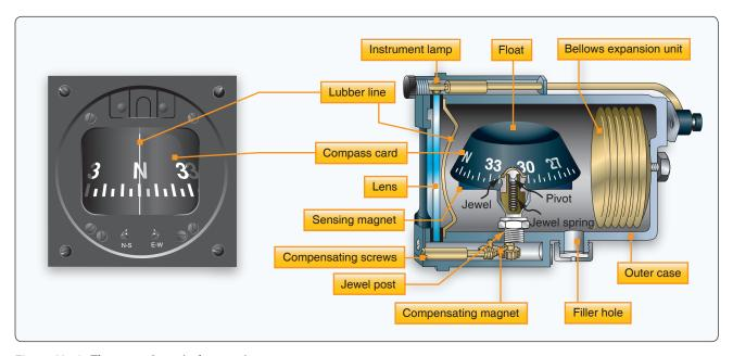
**Figure 10-79.** *The parts of a typical magnetic compass.*
