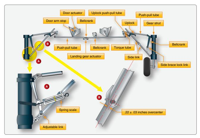
Figure 13-49. Over-center adjustments on a small aircraft main gear.
