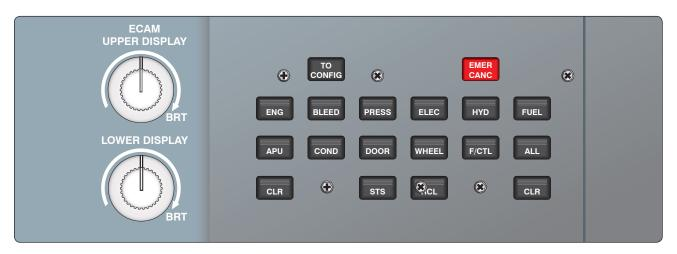
Figure 10-121. An ECAM display control panel.
