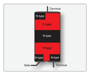
**Figure 11-33.** The semiconductor layering in a triac. A positive or negative gate pulse with respect to the upper terminal allows current to flow through the devise in either direction.
