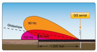
**Figure 11-112.** A glideslope antenna broadcasts radio signals to guide an aircraft vertically to the runway.
