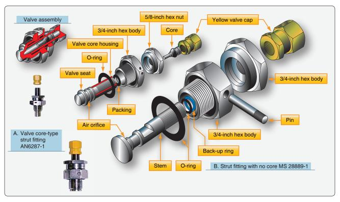
**Figure 13-24.** *Valve core-type (A) and core-free valve fittings (B) are used to service landing gear shock struts.*
