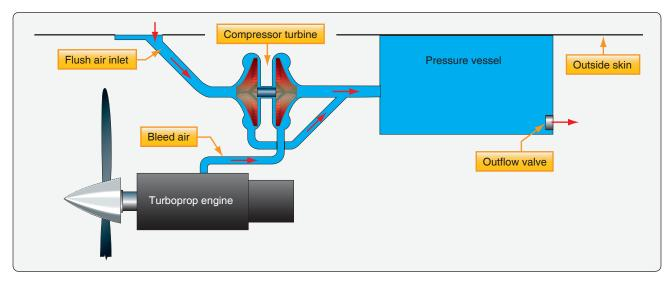
Figure 16-49. A turbo compressor used to pressurize cabins mostly in turboprop aircraft.
