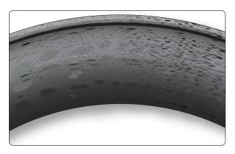
**Figure 13-71.** Bruising is caused by fine particle contamination possibly from a bad seal or improper maintenance of bearing cleanliness. It leaves a less than smooth surface on the bearing cup.
