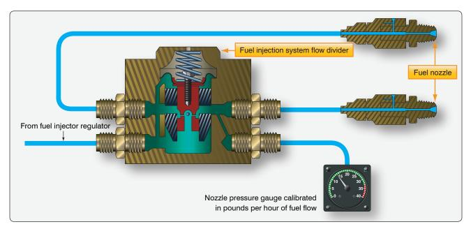
Figure 14-76. The pressure drop across the fuel injector nozzles is used to represent fuel flow in light reciprocating-engine aircraft.
