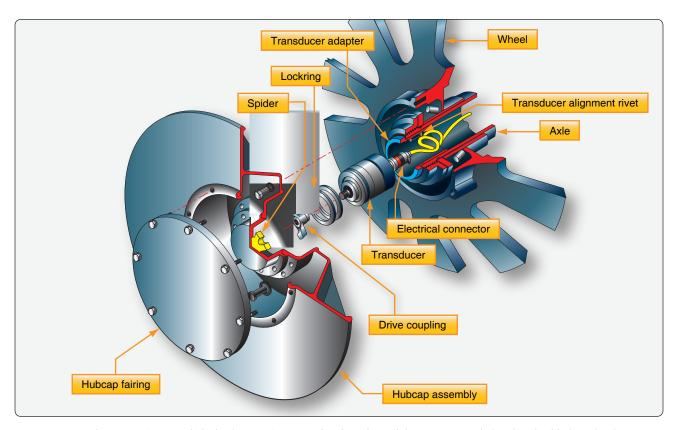
**Figure 13-107.** The stator of an antiskid wheel sensor is mounted in the axle, and the rotor is coupled to the wheel hub spider that rotates with the wheel.
