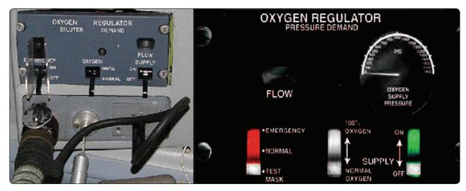
**Figure 16-20.** The two basic types of regulators used in demand flow oxygen systems. The panel below the diluter demand regulator on the left is available for mask hose plug in (left), lanyard mask hanger (center), and microphone plug in (right). Most high performance demand type masks have a microphone built-in.
