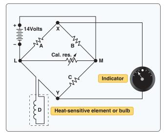
**Figure 10-69.** The internal structure of an electric resistance thermometer indicator features a bridge circuit, galvanometer, and variable resistor, which is outside the indicator in the form of the temperature sensor.
