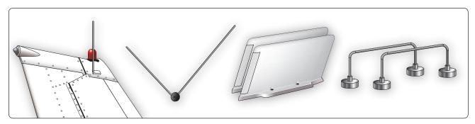
**Figure 11-96.** *V-shaped, horizontally polarized, bi-pole antennas are commonly used for VOR and VOR/glideslope reception. All antenna shown are VOR/glideslope antenna.*
