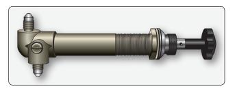
Figure 14-47. This engine primer pump is a hand-operated piston type. It is mounted in the instrument panel and extends through the firewall where fuel intake and delivery lines are attached to the fittings on the left.
