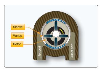
Figure 12-28. Vane-type power pump.
