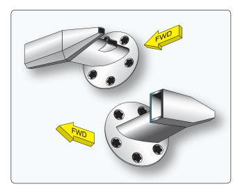
Figure 10-77. Total air temperature (TAT) probes.
