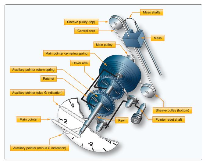
**Figure 10-60.** *The inner workings of a mass-type accelerometer.*
