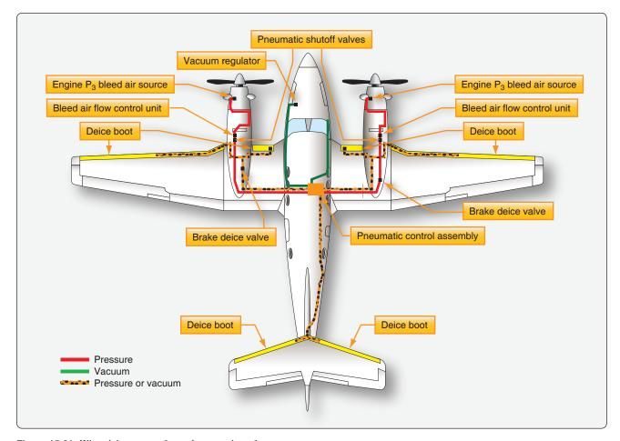
**Figure 15-21.** Wing deice system for turboprop aircraft.
