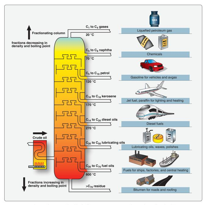
**Figure 14-10.** Petroleum products are produced by distillation. Various fractions condense and are collected at different temperatures that correspond to the height of collection in the distillation tower. As can be seen, there are significant differences between turbine engine fuel and ordinary AVGAS.
