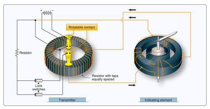
**Figure 10-48.** A lock switch circuit can be added to the basic DC selsyn synchro system when used to indicate landing gear position and up- and down-locked conditions on the same indicator.
