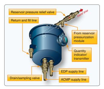
Figure 12-10. Components of an air-pressurized reservoir.
