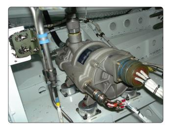
Figure 12-22. Electrically-driven pump.
