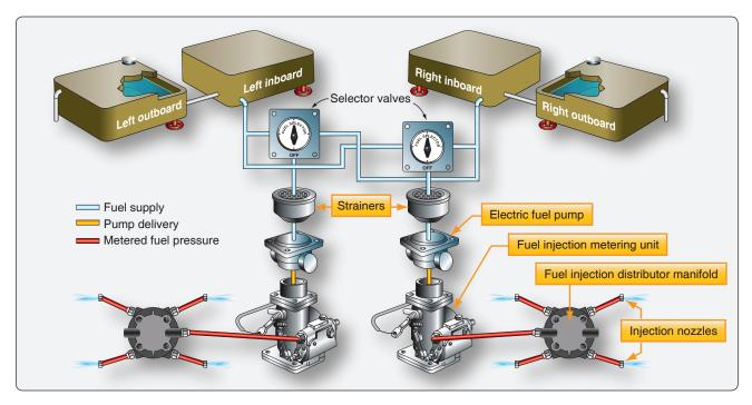
Figure 14-17. A simple high-wing fuel injection fuel system for a light twin reciprocating-engine aircraft.
