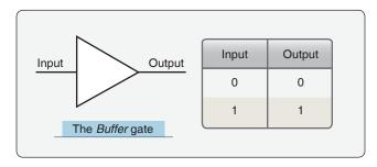
**Figure 11-63.** A buffer or amplifier symbol and the truth table of the buffer, which is actually two consecutive NOT gates.
