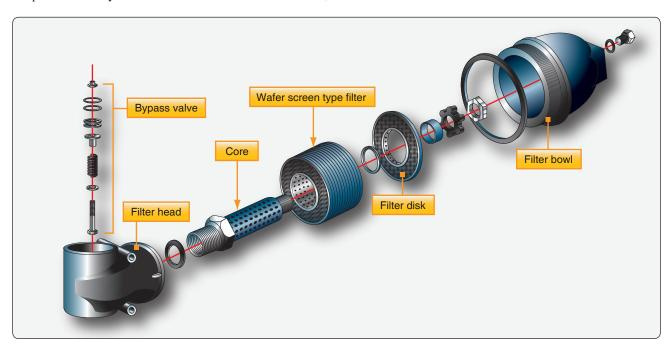
Figure 14-63. A micronic wafer filter uses multiple screen wafers through which fuel must pass to exit the filter through the core. A spring loaded bypass valve in the filter housing unseats when the filter is clogged to continue delivery of fuel.
