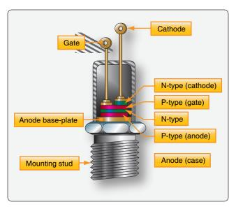
**Figure 11-30.** *Cross-section of a medium-power SCR.*
