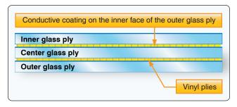
**Figure 15-44.** *Cross-section of a transport category windshield.*
