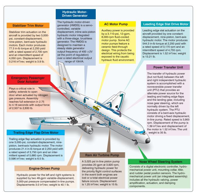
Figure 12-62. *Large aircraft hydraulic systems*.
