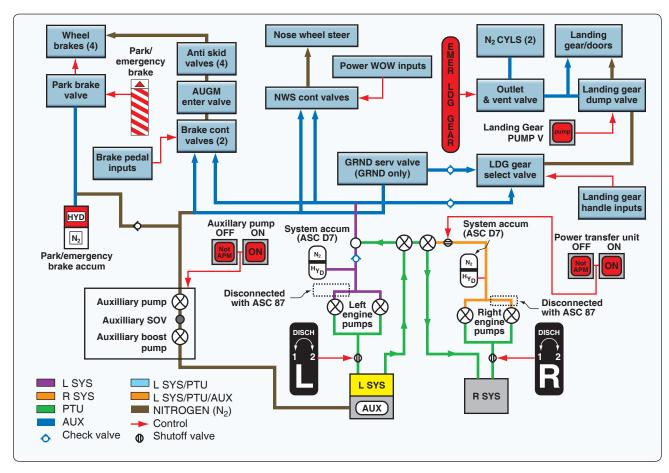
**Figure 12-76.** *Pneumatic emergency landing gear extension system.*
