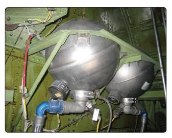
**Figure 17-12.** Built-in non-portable fire extinguisher containers (HRD bottles) on an airliner.
