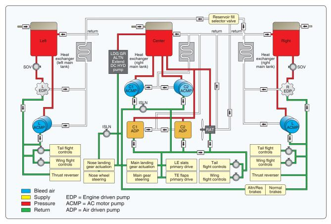
Figure 12-66. A Boeing 777 hydraulic system.
