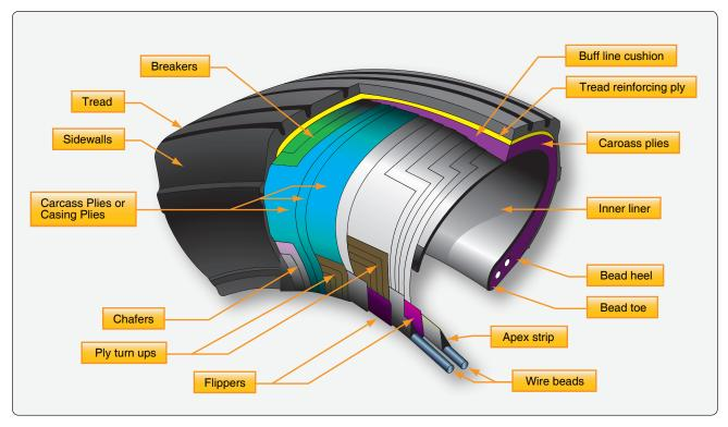
Figure 13-130. Construction nomenclature of an aircraft tire.
