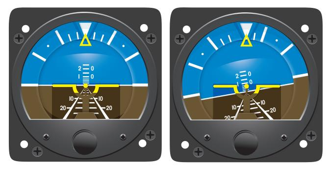
Figure 10-100. A typical vacuum-driven attitude indicator shown with the aircraft in level flight (left) and in a climbing right turn (right).
