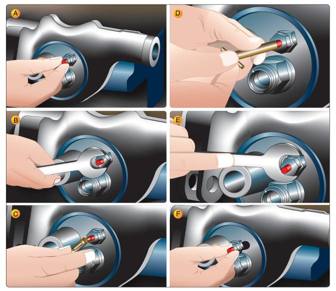
**Figure 13-25.** Steps in servicing a landing gear shock strut include releasing the air from the strut and removing the service valve from the top of the strut to permit the introduction of hydraulic fluid. Note that the strut is illustrated horizontally. On an actual aircraft installation, the strut is serviced in the vertical position (landing gear down).
