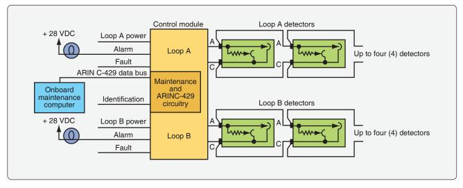
Figure 17-8. Aircraft detection system control module.
