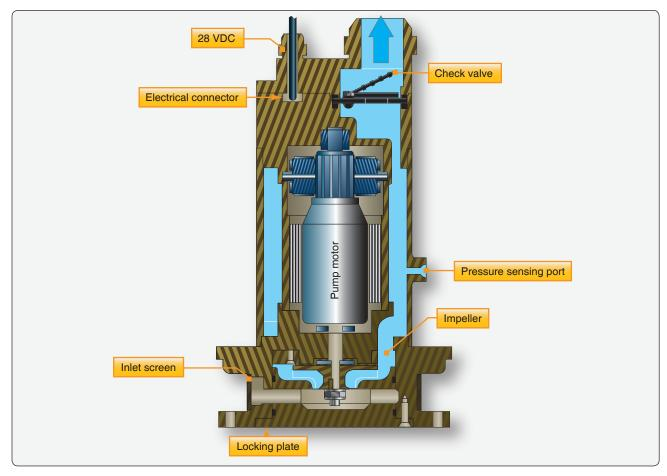
**Figure 14-49.** The internal workings of a centrifugal fuel boost pump. Fuel is drawn into the center of the impeller through a screen. It is moved to the outside of the case by the impeller and out the fuel outlet tube.
