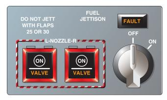
Figure 14-4. The fuel jettison panel on a Boeing 767.
