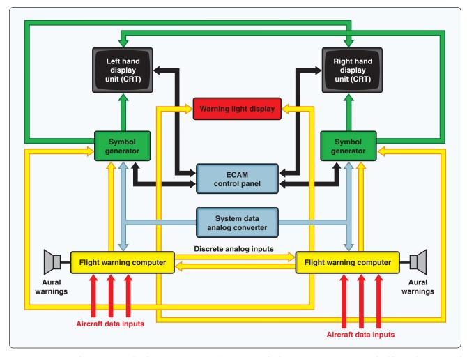
**Figure 10-120.** An electronic centralized aircraft monitor (ECAM) system displays aircraft system status, checklists, advisories, and warnings on a pair of controllable monitors.
