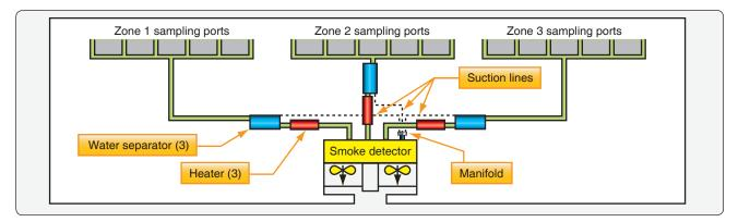
Figure 17-20. Smoke detector system.
