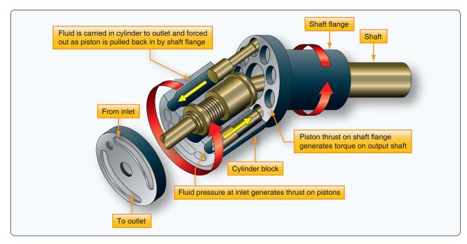
Figure 12-55. Bent axis pistion motor.
