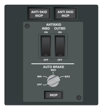
**Figure 13-105.** *Antiskid switches in the cockpit.*
