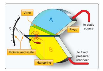
**Figure 10-41.** A variometer uses differential pressure to indicate vertical speed. A rotating vane separating two chambers (one with static pressure, the other with a fixed pressure reservoir), moves the pointer as static pressure changes.
