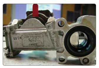
Figure 14-40. This motor-operated gate valve has a red position indicating lever that can be used by maintenance personnel to identify the position of the valve. The lever can be moved by the technician to position the valve.
