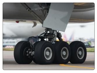
Figure 13-9. Triple bogie main landing gear assembly on a Boeing
