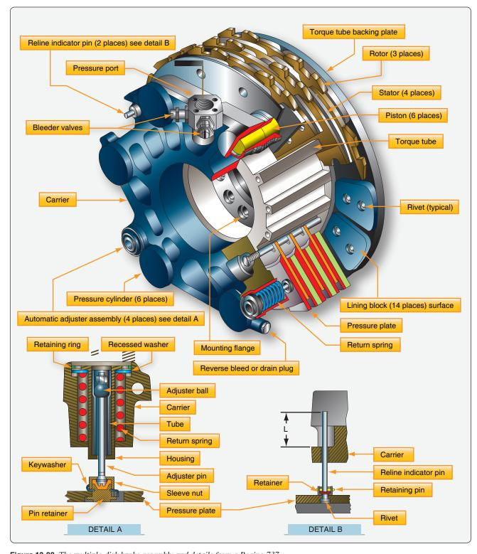
$\textbf{Figure 13-88.} \ \textit{The multiple-disk brake assembly and details from a Boeing 737.}$
