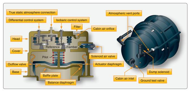
Figure 16-54. An all-pneumatic cabin pressure regulator and outflow valve.
