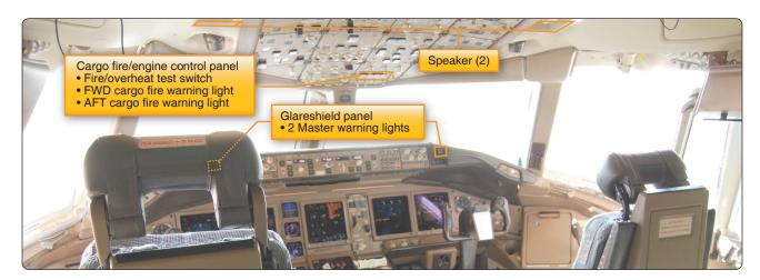
Figure 17-18. Cargo fire detection warning.
