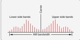
**Figure 11-82.** The bandwidth of an AM signal contains the carrier wave, the carrier wave plus the information signal frequencies, and the carrier wave minus the information signal frequencies.
