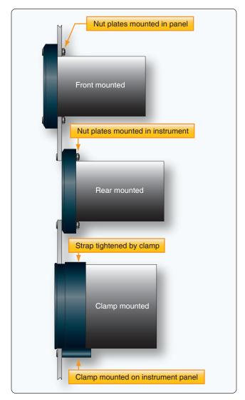
**Figure 10-135.** *Instrument mounts—flanged (top and middle) and flangeless (bottom).*
