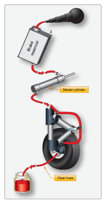
**Figure 13-119.** Arrangement for top down or gravity bleeding of aircraft brakes.
