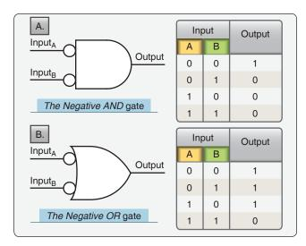
Figure 11-69. The NEGATIVE AND gate symbol and its truth table (A) and the NEGATIVE OR gate symbol and truth table (B). The inputs are inverted in the NEGATIVE gates.
