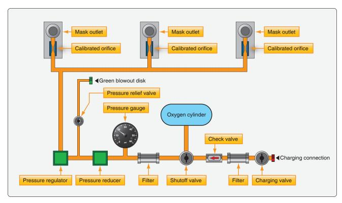
Figure 16-13. Continuous flow oxygen system found on small to medium size aircraft.
