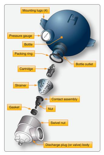
**Figure 17-30.** *Components of fire extinguisher container.*
