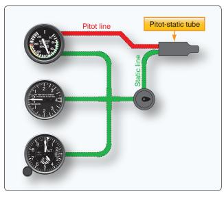
**Figure 10-22.** A simple pitot-static system is connected to the primary flight instruments.
