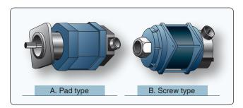
**Figure 10-56.** *Different types of tach generators.*
