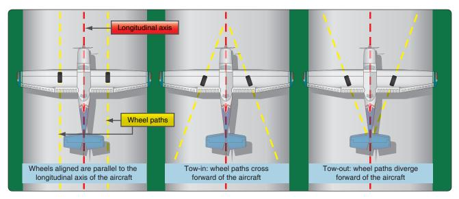
Figure 13-28. Wheel alignment on an aircraft.
