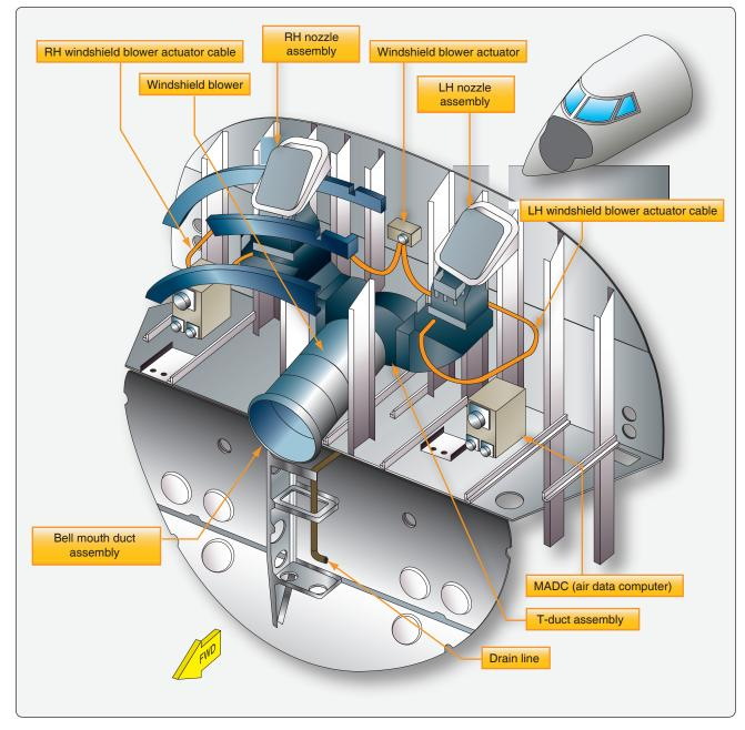
**Figure 15-43.** *Windshield rain and frost removal system.*
