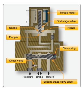
**Figure 13-110.** An antiskid control valve uses a torque motor controlled flapper in the first stage of the valve to adjust pressure on a spool in the second stage of the valve to build or relieve pressure to the brake.
