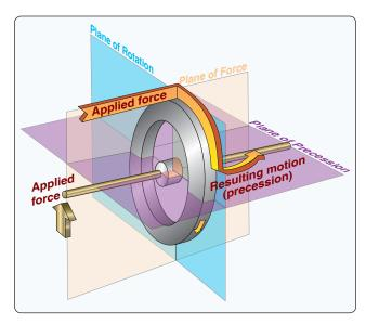
**Figure 10-95.** When a force is applied to a spinning gyroscope, it reacts as though the force came from 90° further around the rotor in the direction it is spinning. The plane of the applied force, the plane of the rotation, and the plane in which the gyro responds (known as the plane of precession), are all perpendicular to each other.
