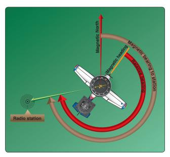
**Figure 11-103.** Older ADF indicators have nonrotating azimuth cards.  $0^{\circ}$  is fixed at the top of the instrument and the pointer always indicates the relative bearing to the ADF transmission antenna. To fly to the station, the pilot turns the aircraft until the ADF pointer indicates  $0^{\circ}$ .
