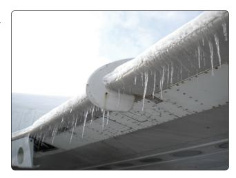
**Figure 15-1.** *Formation of ice on aircraft leading edge.*
