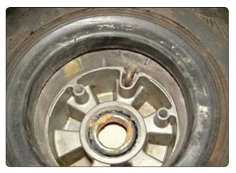
**Figure 13-157.** *Mounting a tube type tire with the tube valve stem positioned to pass through the outboard wheel half.*
