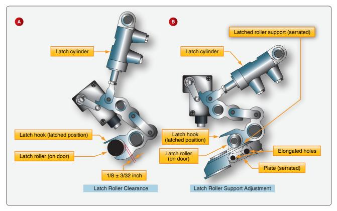
**Figure 13-47.** *Main landing gear door latch roller clearance measurement and adjustment.*
