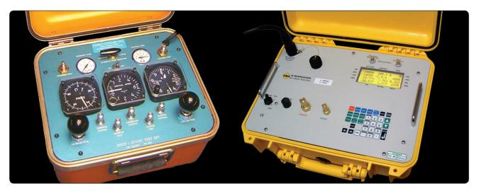
Figure 10-138. An analog pitot-static system test unit (left) and a digital pitot static test unit (right).
