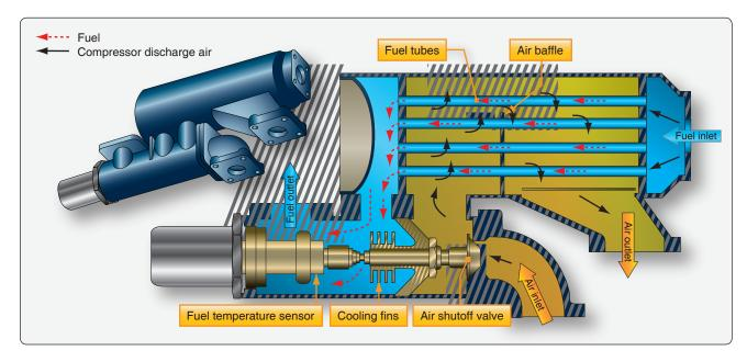
Figure 14-65. An air-fuel heat exchanger uses engine compressor bleed air to warm the fuel on many turbine engine powered aircraft.
