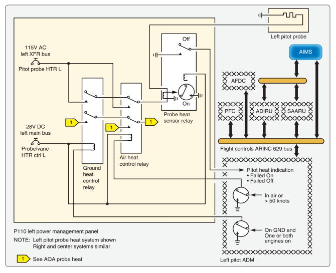
Figure 15-15. Pitot probe heat system.
