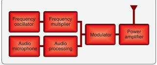
Figure 11-84. Block diagram of a basic radio transmitter.
