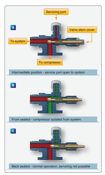
**Figure 16-85.** Compressor isolation valves isolate the compressor for maintenance or replacement. They also allow normal operation and servicing of the vapor cycle air conditioning system with refrigerant.
