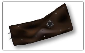
Figure 14-31. A bladder fuel tank for a light aircraft.
