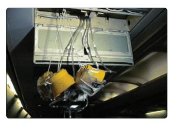
**Figure 16-15.** A passenger service unit (psu) is hinged over each row of seats in an airliner. Four yellow continuous flow oxygen masks are shown deployed. They are normally stored behind a separate hinged panel that opens to allow the masks to fall from the PSU for use.
