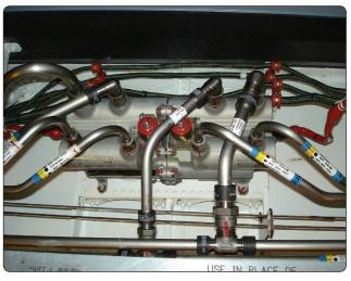
Figure 12-35. Four-way servo control valve.
