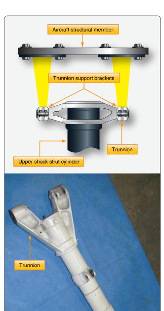
**Figure 13-32.** The trunnion is a fixed structural support that is part of or attached to the upper strut cylinder of a landing gear strut. It contains bearing surfaces so the gear can retract.
