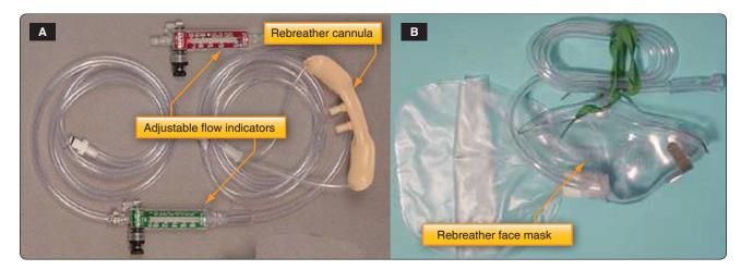
**Figure 16-14.** A rebreather cannula (A) and rebreather bag (B) capture exhaled oxygen to be inhaled on the next breath. This conserves oxygen by permitting lower flow rates in continuous flow systems. The red and green devices are optional flow indicators that allow the user to monitor oxygen flow rate. The type shown also contains needle valves for final regulation of the flow rate to each user.
