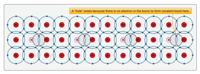
**Figure 11-18.** The lattice of boron doped silicon contains holes where the three boron valence shell electrons fail to fill in the combined valence shells to the maximum of eight electrons. This is known as *P-type semiconductor material* or acceptor material.
