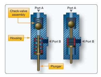
Figure 12-40. Mechanically operated sequence valve.
