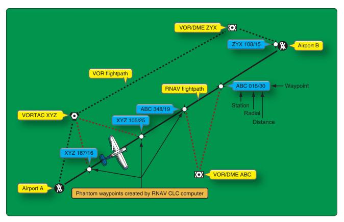
**Figure 11-123.** The pilot uses the aircraft's course deviation indicator to fly to and from RNAV phantom waypoints created by computer. This allows direct routes to be created and flown rather than flying from VOR to VOR.
