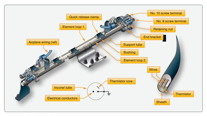
Figure 17-4. Kidde continuous-loop system.
