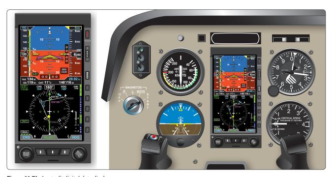
Figure 11-71. A retrofit digital data display.
