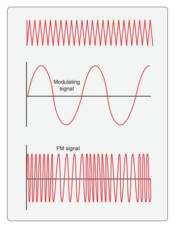
Figure 11-81. A frequency modulated (FM) carrier wave retains the consistent amplitude of the AC sign wave. It encodes the unique information signal with slight variations to the frequency of the carrier wave. These variations are shown as space variations between the peaks and valleys of the wave on an oscilloscope.
