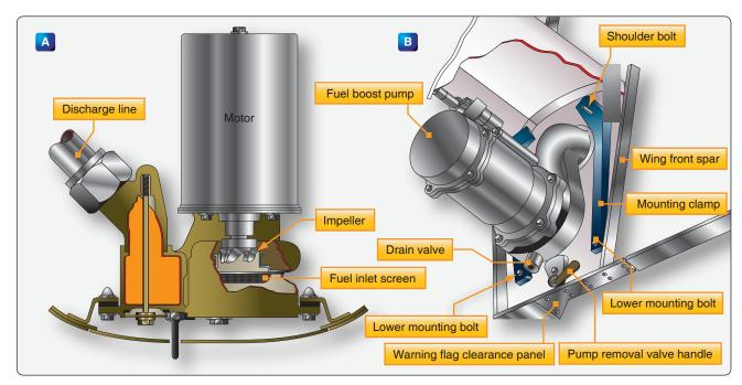
**Figure 14-48.** A centrifugal fuel boost pump can be submersed in the fuel tank (A) or can be attached to the outside of the tank with inlet and outlet plumbing extending into the tank (B). The pump removal valve handle extends below the warning flag clearance panel to indicate the pump inlet is closed.
