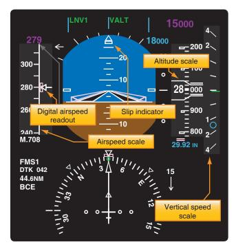
**Figure 10-119.** An EFIS EADI displays an airspeed scale to the left of the horizon sphere and an altimeter and vertical speed scale to the right. The slip indicator is the small rectangle under the direction triangles at the top. This EFIS display presents all of the flight information in the conventional cockpit basic T.
