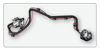
Figure 17-6. Pneumatic dual fire/overheat detector assembly.
