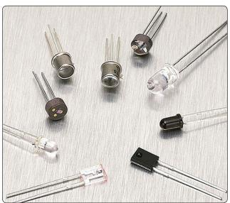
Figure 11-40. Phototransistors.
