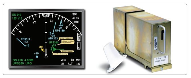
Figure 11-137. A cockpit display of ADS-B generated targets (left) and an ADS-B airborne receiver with antenna (right).
