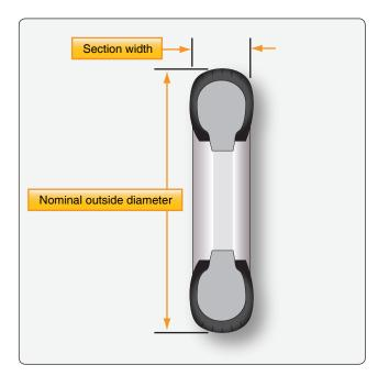
Figure 13-126. A Type VII aircraft tire is identified by its twonumber designation. The first number represents the tire's overall diameter in inches and the second number represents the section width in inches. Type VII designators separate the first and second number an "X." For example: 26 X 6.6 identifies a tire that is 26 inches in diameter with a 6.6-inch nominal width.
