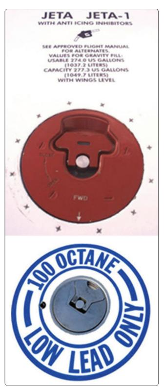
**Figure 14-97.** All entry points of fuel into the aircraft are marked with the type of fuel to be used. Never introduce any other fuel into the aircraft other than that which is specified.
