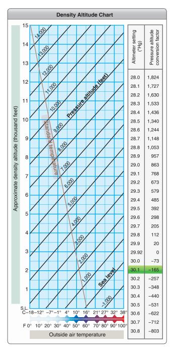
**Figure 10-36.** The effect of air temperature on aircraft performance is expressed as density altitude.
