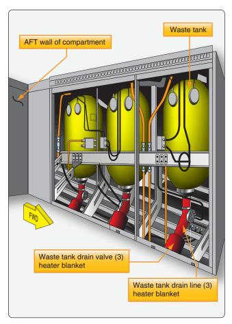
**Figure 15-48.** *Waste water tanks and heater blankets.*
