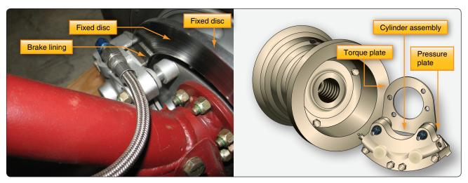
**Figure 13-81.** A Cleveland brake on a light aircraft is a fixed-disc brake. It allows the brake caliper to move laterally on anchor bolts to deliver even pressure to each side of the brake disc.
