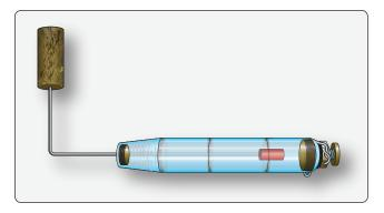
**Figure 14-67.** *A float-type sight gauge fuel quantity indicator.*
