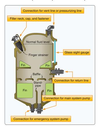
Figure 12-8. Nonpressurized reservoir.
