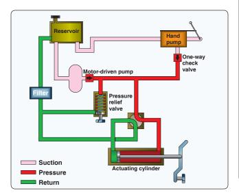
Figure 12-2. Basic hydraulic system.
