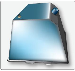
$\textbf{Figure 14-30.} \ A\ composite\ tank\ from\ a\ Challenger\ ultralight\ aircraft.$
