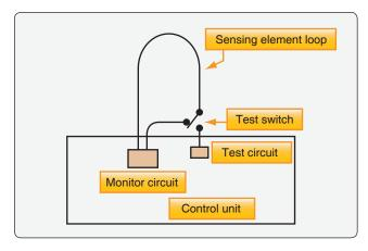
Figure 17-5. Continuous loop fire detection system test circuit.
