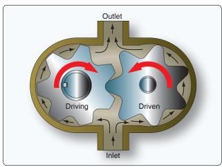
Figure 12-23. Gear-type power pump.
