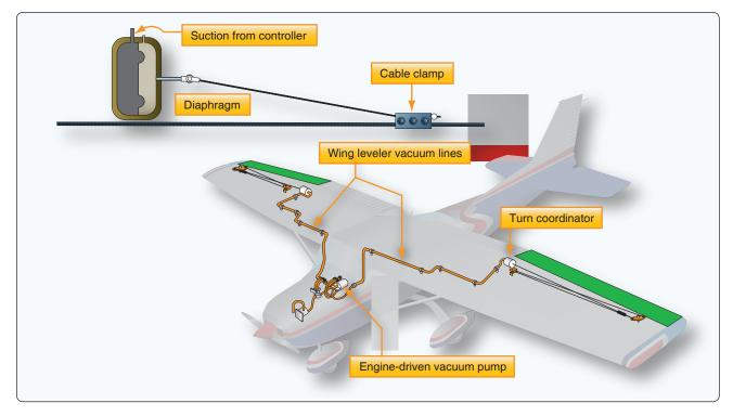
Figure 10-107. The wing leveler system on a small aircraft is a vacuum-operated single-axis autopilot. Only the ailerons are controlled. The aircraft's turn coordinator is the sensing element. Vacuum from the instrument vacuum system is metered to the diaphragm cable actuators to move the ailerons when the turn coordinator senses roll.
