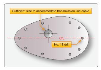
**Figure 11-161.** *A typical antenna mounting template.*
