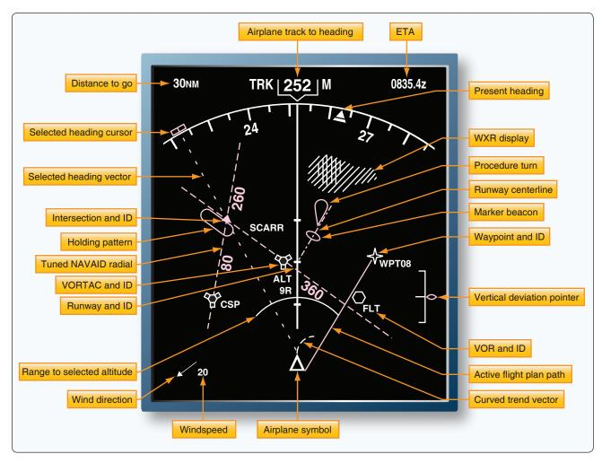
**Figure 10-116.** An EHSI presents navigational information for the entire flight. The pilot selects the mode most useful for a particular phase of flight, ranging from navigational planning to instrument approach to landing. The MAP mode is used during most of the flight.
