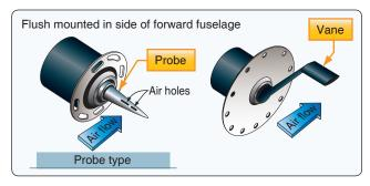
Figure 10-64. A slotted AOA probe and an alpha vane.
