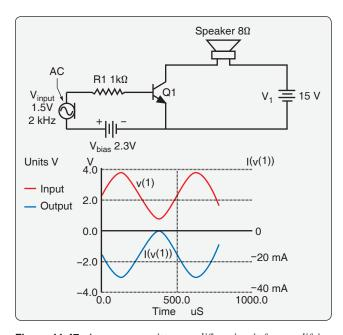
Figure 11-47. A common-emitter amplifier circuit for amplifying an AC microphone signal to drive a speaker (top) and the graph of the output signal showing a 180 degree shift in phase (bottom).
