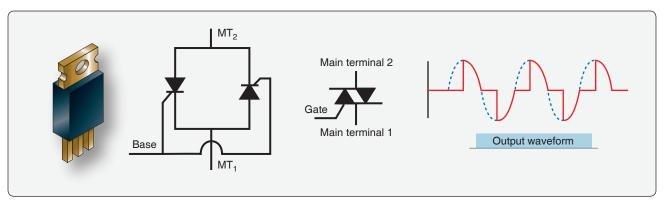
Figure 11-32. A triac is a controlled semiconductor device that allows current flow in both directions.
