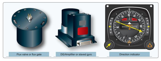
Figure 10-82. Components used to prvide direction indication.
