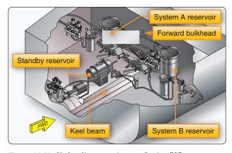
Figure 12-63. Hydraulic reservoirs on a Boeing 737.
