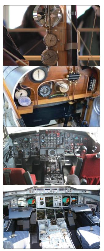
**Figure 10-1.** From top to bottom: instruments of the Wright Flyer, instruments on a World War Lera aircraft, a late 1950s/early 1960s Boeing 707 airliner cockpit, and an Airbus A380 glass cockpit.
