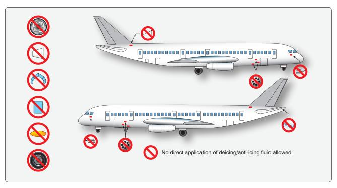
**Figure 15-39.** *No direct application of deicing/anti-icing fluid allowed.*
