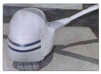
**Figure 13-11.** Wheel fairings, or pants, and low profile struts reduce parasite drag on fixed gear aircraft.
