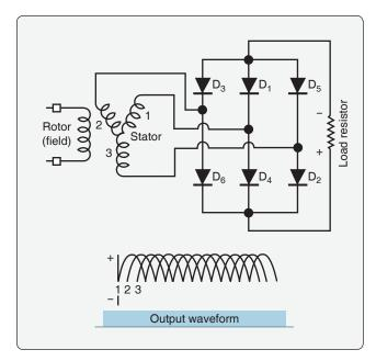
Figure 11-46. A six-diode, three-phase AC rectifier.
