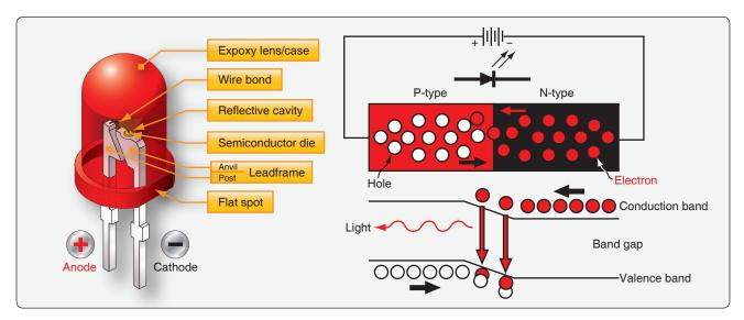
**Figure 11-42.** A close up of a single LED (left) and the process of a semi-conductor producing light by electrons dropping into holes and giving off energy (right). The symbol for a light emitting diode is the diode symbol with two arrows pointing away from the junction.
