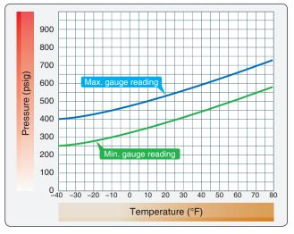
**Figure 17-29.** Fire extinguisher container pressure-temperature chart.
