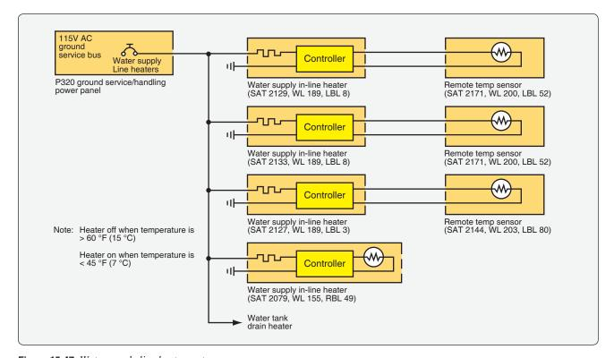
**Figure 15-47.** Water supply line heater system.
