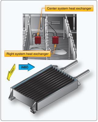
Figure 12-51. *Hydraulic heat exchanger*.
