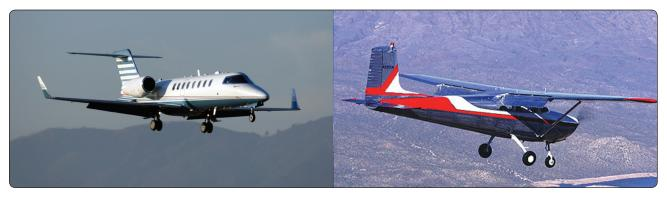
Figure 13-6. Tricycle-type landing gear with dual main wheels on a Learjet (left) and a Cessna 172, also with tricycle gear (right).
