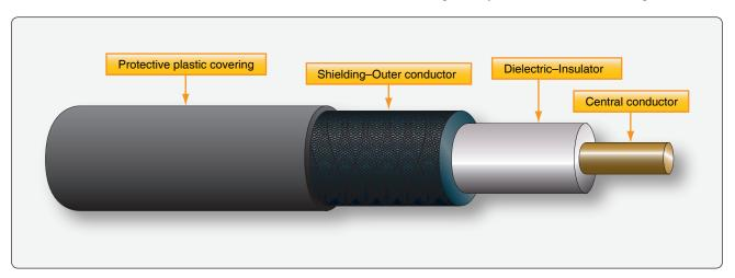
Figure 11-94. Coaxial cable is used as the transmission line between an antenna and its transmitters and/or receiver.
