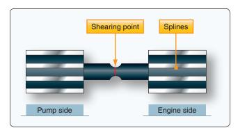
Figure 12-26. Hydraulic pump shear shaft.
