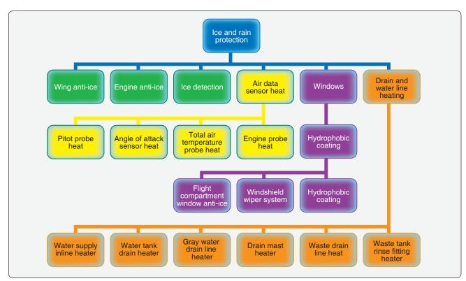
**Figure 15-3.** *Ice and rain protection systems.*
