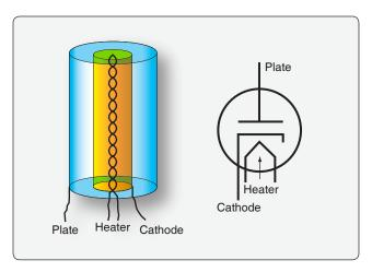
**Figure 11-5.** A vacuum tube diode contains a cathode, heater, and plate. Note that the arrow formed in the symbol for the heater points to the direction of electron flow.
