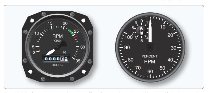
$\textbf{Figure 10-52.} \ A \ tachometer for \ a \ reciprocating \ engine \ is \ calibrated \ in \ rpm. \ A \ tachometer for \ a \ turbine \ engine \ is \ calculated \ in \ percent \ of \ rpm.$
