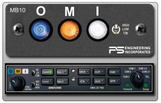
**Figure 11-116.** Various marker beacon instrument panel display lights.
