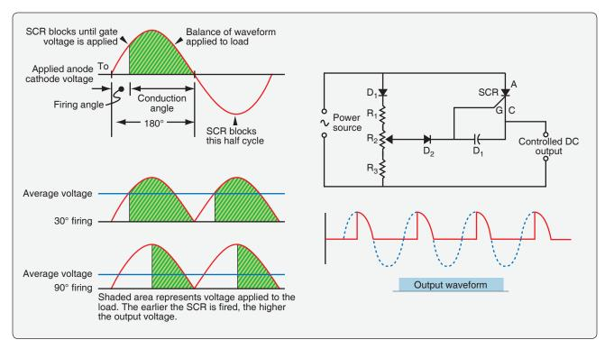
**Figure 11-31.** Phase control is a key application for SCR. By limiting the percentage of a full cycle of AC voltage that is applied to a load, a reduced voltage results. The firing angle or timing of a positive voltage pulse through the SCR's gate latches the device open allowing current flow until it drops below the holding current, which is usually at or near zero voltage as the AC cycle reverses.
