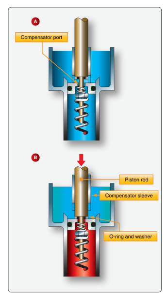
Figure 13-95. A common master cylinder with built-in reservoir is shown. Illustration A depicts the master cylinder when the brakes are off. The compensating port is open to allow fluid to expand into the reservoir should temperature increase. In B, the brakes are applied. The piston rod-end seal covers the compensating port as it contacts the piston head.
