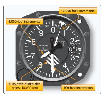
**Figure 10-32.** A sensitive altimeter with three pointers and a cross-hatched area displayed during operation below 10,000 feet.
