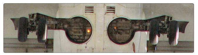
**Figure 13-12.** The retractable gear of a Boeing 737 fair into recesses in the fuselage. Panels attached to the landing gear provide smooth airflow over the struts. The wheel assemblies mate with seals to provide aerodynamic flow without doors.
