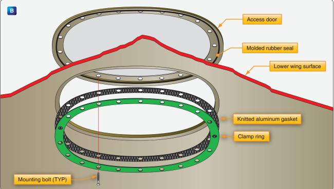
Figure 14-33. Fuel tank access panel locations on a Boeing 737 (A), and typical fuel tank access panel seals (B).
