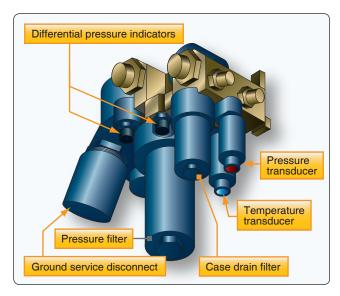
Figure 12-15. Filter module components.
