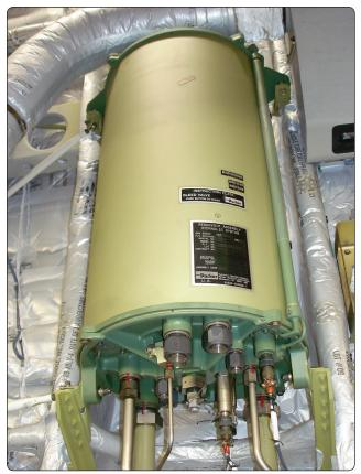
Figure 12-9. Air-pressurized reservoir.
