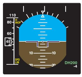
**Figure 11-141.** The decision height, DH200, in the lower right corner of this EADI display uses the radar altimeter as the source of altitude information.
