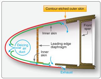
Figure 15-8. Heated wing leading edge.
