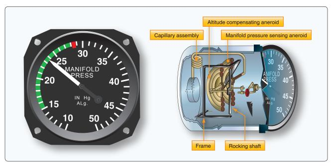
Figure 10-15. An analog manifold pressure indicator instrument dial calibrated in inches of mercury (left). The internal workings of an analog manifold pressure gauge are shown on the right. Air from the intake manifold surrounds the aneroid causing it to deflect and indicate pressure on the dial through the use of linkage to the pointer (right).
