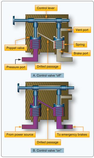
Figure 12-72. Pneumatic control valve.
