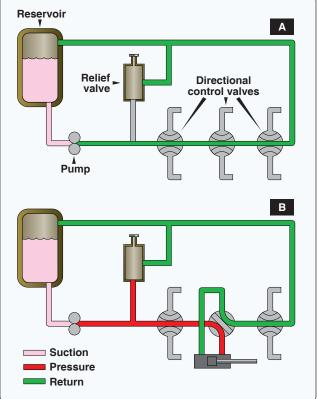
Figure 12-3. Open center hydraulic system.
