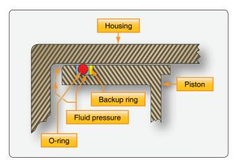
**Figure 13-121.** Back-up rings are used to keep O-rings from extruding into the space between the piston and the cylinder. They are positioned on the side of the O-ring away from the fluid pressure.
