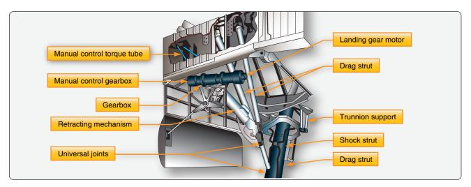
Figure 13-34. A geared electric motor landing gear retraction system.
