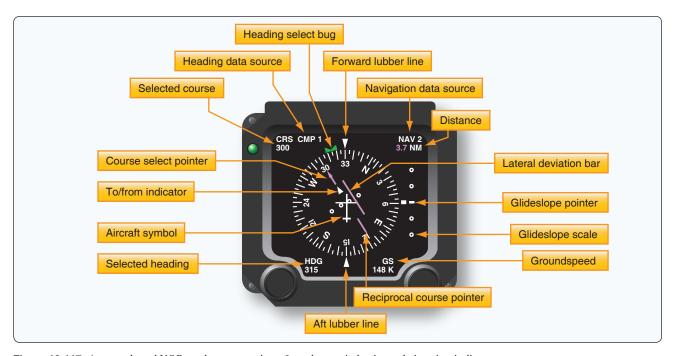
**Figure 10-117.** Approach and VOR mode presentation of an electronic horizontal situation indicator.
