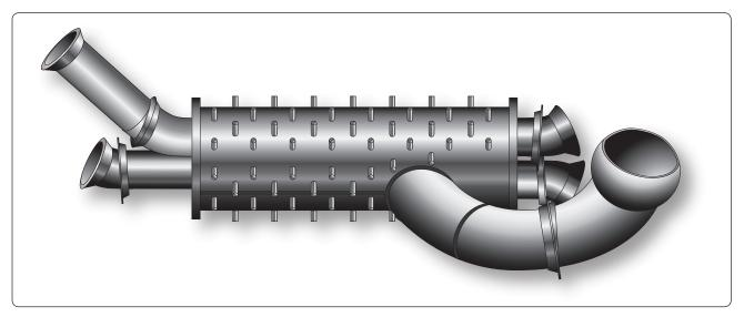
**Figure 16-98.** An exhaust manifold with its shroud removed showing numerous welded studs used to increase heat transfer from the exhaust to the ambient air going to the cabin.
