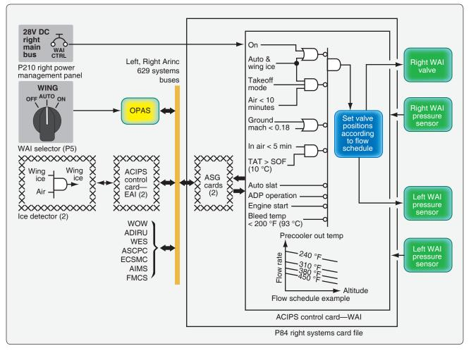
Figure 15-12. WAI inhibit logic schematic.
