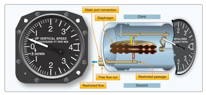
**Figure 10-39.** The VSI is a differential pressure gauge that compares free-flowing static air pressure in the diaphragm with restricted static air pressure around the diaphragm in the instrument case.
