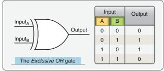
**Figure 11-68.** An EXCLUSIVE OR gate symbol and its truth table, which is similar to an OR gate but excludes output when both inputs are the same.
