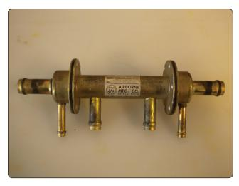
**Figure 15-28.** A manifold assembly used in multiengine aircraft deice systems.
