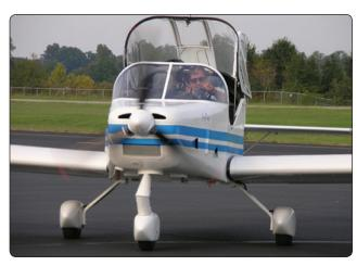
**Figure 13-13.** Non-shock absorbing struts made from steel, aluminum, or composite material transfer the impact forces of landing to the airframe at a non-damaging rate.
