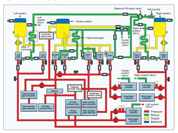
Figure 12-6. Large commercial aircraft hydraulic system.
