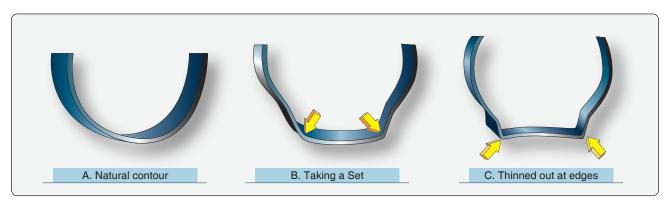
**Figure 13-152.** During inspection, an aircraft tire tube should retain its natural contour. Tubes with thinned areas or that have taken a set should be discarded and replaced.
