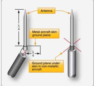
Figure 11-92. On a metal-skinned aircraft, a ½ wavelength Marconi antenna is used. The skin is the ground plane that creates the 2nd quarter of the antenna required for resonance (left). On a non-metallic-skinned aircraft, wires, conductive plates or strips equal in length to the antenna must be installed under the skin to create the ground plane (right).
