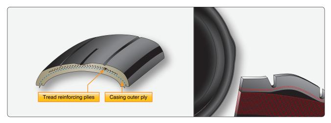
**Figure 13-141.** Bulges and tread separation are cause for removal of a tire from service.
