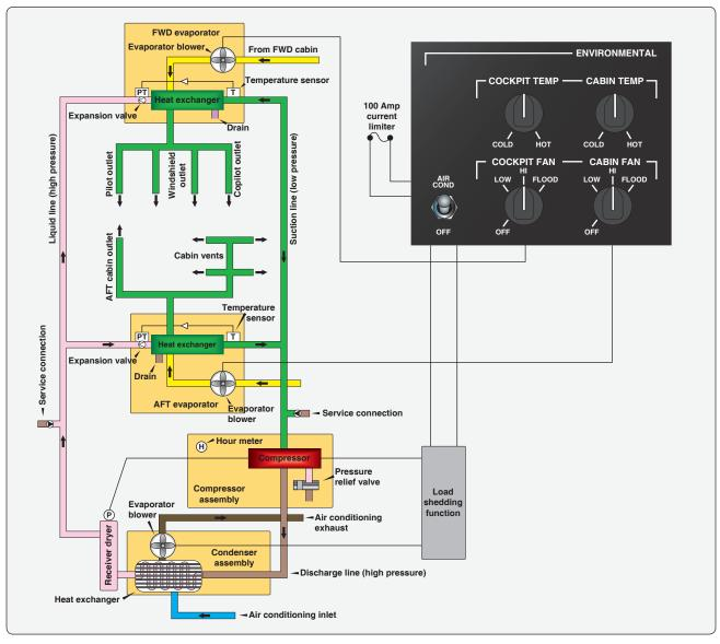
**Figure 16-80.** The vapor cycle air conditioning system on a Cessna Mustang has two evaporators, one for the cockpit and one for the cabin. Each evaporator assembly contains the evaporator, a blower, a thermal expansion valve and the temperature feedback line from the outlet of the evaporator to the expansion valve.
