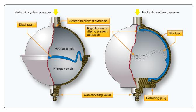
**Figure 12-49.** A spherical accumulator with diaphragm (left) and bladder (right). The dotted lines in the right drawing depict the bladder when the accumulator is charged with both hydraulic system fluid and nitrogen preload.
