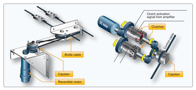
Figure 10-109. A reversible motor with capstan and bridle cable (left), and a single-direction constant motor with clutches that drive the output shafts and control cable in opposite directions (right).
