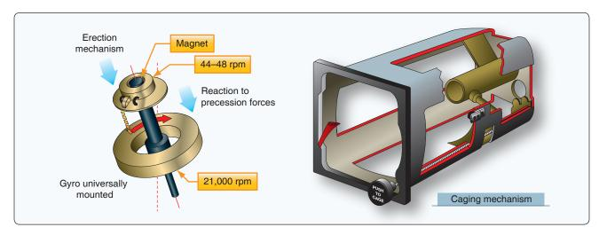
**Figure 10-102.** *Erecting and caging mechanisms of an electric attitude indicator.*
