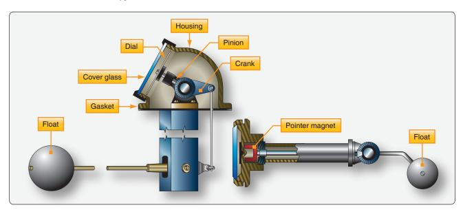
Figure 14-68. Simple mechanical fuel indicators used on light aircraft with fuel tanks in close proximity to the pilot.
