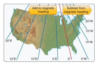
**Figure 10-80.** Aircraft located along the agonic line have  $0^{\circ}$  of variation between magnetic north and true north. Locations on and between the isogonic lines require addition or subtraction, as shown, to magnetic indications to arrive at a true geographic direction.
