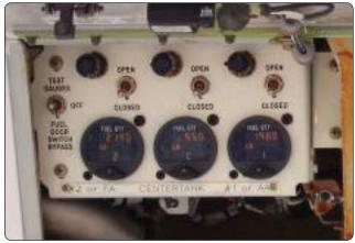
**Figure 14-106.** This panel at the pressure refueling station has valve position switches and quantity gauges to be used during refueling. Valve open position lights are adjacent to the switches for each tank.
