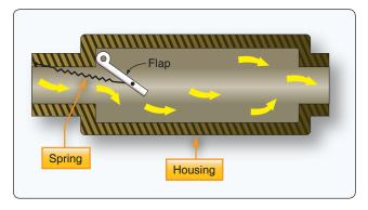
Figure 12-73. Flap-type pneumatic check valve.
