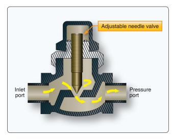
Figure 12-75. Variable pneumatic restrictor.
