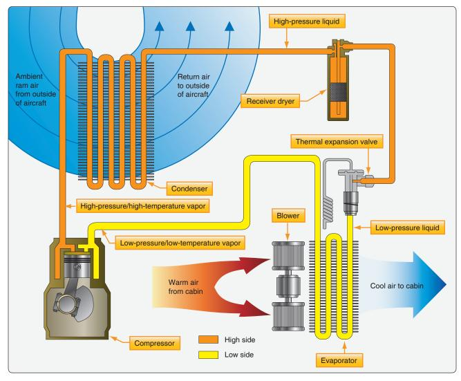
**Figure 16-74.** A basic vapor cycle air conditioning system. The compressor and the expansion valve are the two components that separate the low side from the high side of the cycle. This figure illustrates this division. Refrigerant on the low side is characterized as having low pressure and temperature. Refrigerant on the high side has high pressure and temperature.
