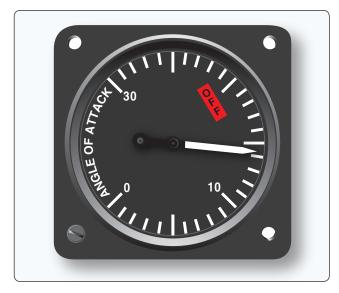
Figure 10-63. Angle of attack indicator.
