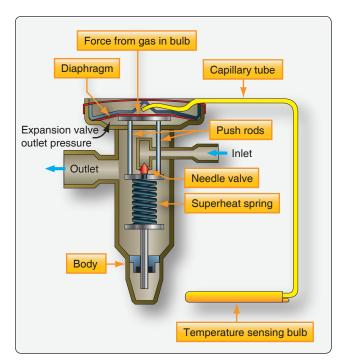
Figure 16-77. An internally equalized expansion valve.
