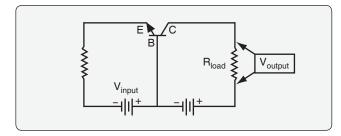
Figure 11-52. A common-base amplifier circuit for DC current.
