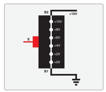
Figure 11-35. The voltage gradient in a UJT.
