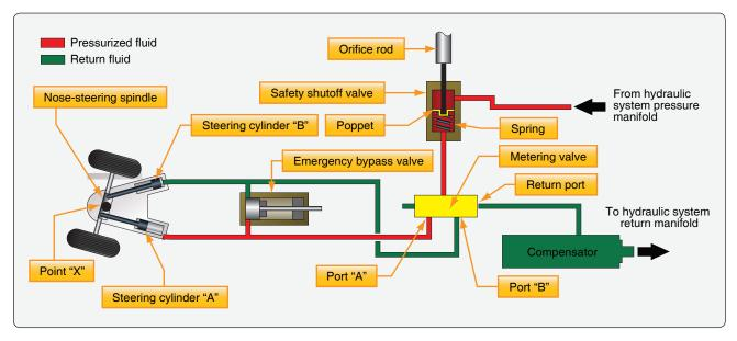
**Figure 13-52.** *Hydraulic system flow diagram of large aircraft nose wheel steering system.*
