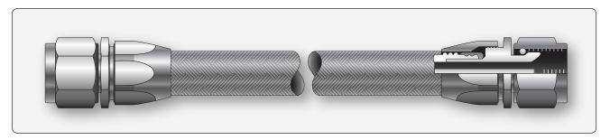
Figure 14-35. A braided stainless steel exterior fuel line with fittings.
