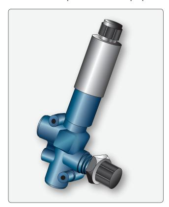
Figure 15-26. A solenoid operated deice control valve.
