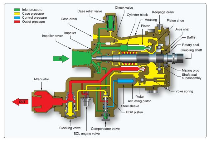
Figure 12-29. Variable displacement pump.
