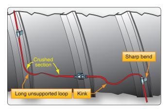
Figure 17-25. Sensing element defects.
