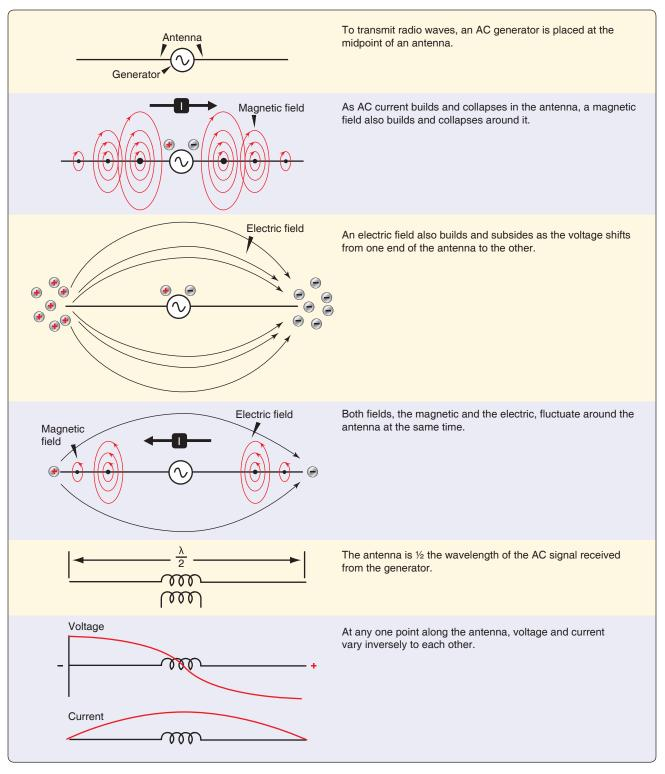
**Figure 11-76.** Radio waves are produced by applying an AC signal to an antenna. This creates a magnetic and electric field around the antenna. They build and collapse as the AC cycles. The speed at which the AC cycles does not allow the fields to completely collapse before the next fields build. The collapsing fields are then forced out into space as radio waves.
