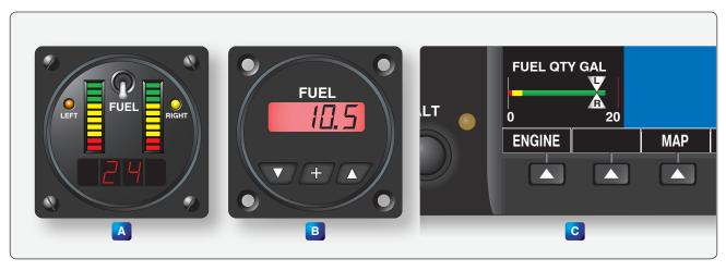
**Figure 14-70.** Digital fuel quantity gauges that work off of variable resistance from the tank unit are shown in A and B. The fuel quantity indication of a Garmin G-1000 flat screen display is shown in C.
