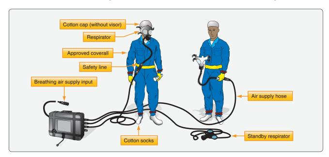
Figure 14-91. Wear a nonstatic protective suit and respirator when entering an integral fuel tank for inspection or repair.
