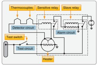
Figure 17-2. Thermocouple fire warning circuit.
