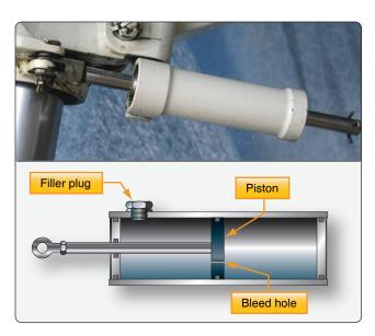
Figure 13-54. A shimmy damper on the nose strut of a small aircraft. The diagram shows the basic internal arrangement of most shimmy dampers. The damper in the photo is essentially the same except the piston shaft extends through both ends of the damper cylinder body.
