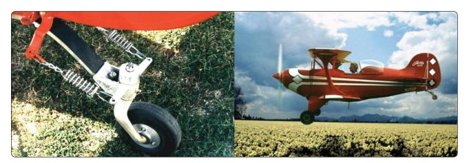
**Figure 13-4.** *The steerable tail wheel of a Pitts Special.*
