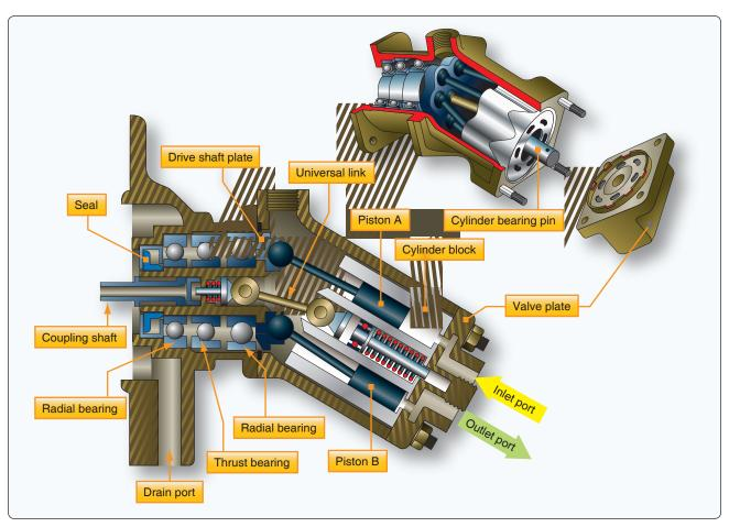
Figure 12-27. Bent axis piston pump.
