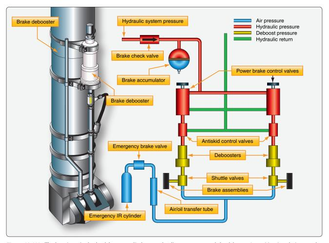
**Figure 13-103.** The location of a brake debooster cylinder on a landing gear strut and the debooster's position in relation to other components of a power brake system.
