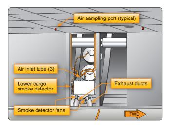
Figure 17-19. Smoke detector installation.
