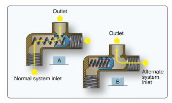
**Figure 12-47.** A spring-loaded piston-type shuttle valve in normal configuration (A) and with alternate/emergency supply (B).
