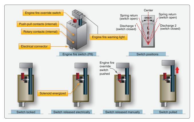
Figure 17-17. Engine fire switch operation.
