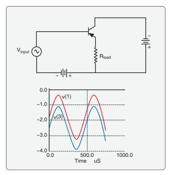
**Figure 11-50.** A common-collector amplifier circuit with a PNP transistor has the same characteristics as that of a common-collector amplifier with a NPN transistor except for reversed voltage polarities and current direction.
