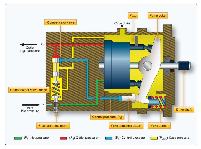
Figure 12-30. Normal pumping mode.
