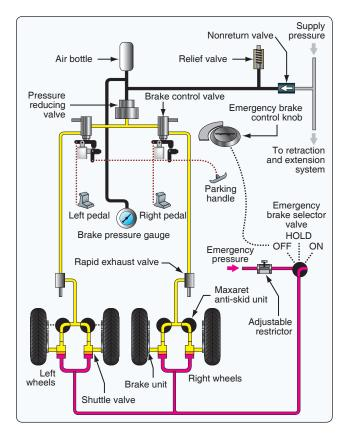
Figure 12-71. Pneumatic brake system.
