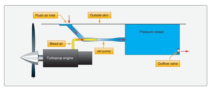
$\textbf{Figure 16-48.} \ \textit{A jet pump flow multiplier ejects bleed air into a venturi which draws air for pressurization from outside the aircraft.}$
