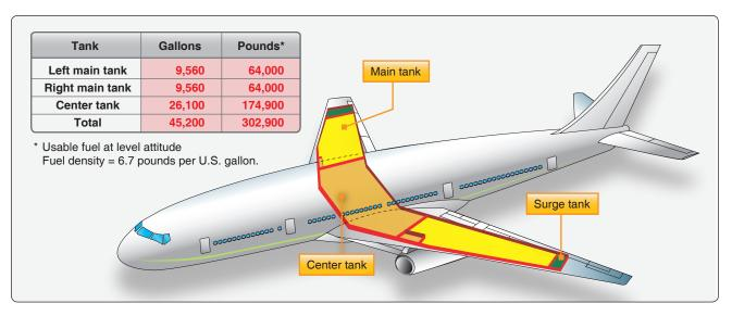
Figure 14-19. Boeing 777 fuel tank locations and capacities.
