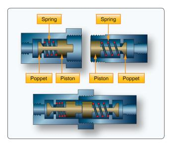
Figure 12-42. A hydraulic quick-disconnect valve.
