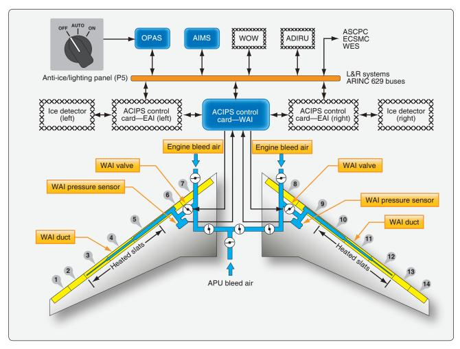
Figure 15-9. Wing leading edge slat anti-ice system.
