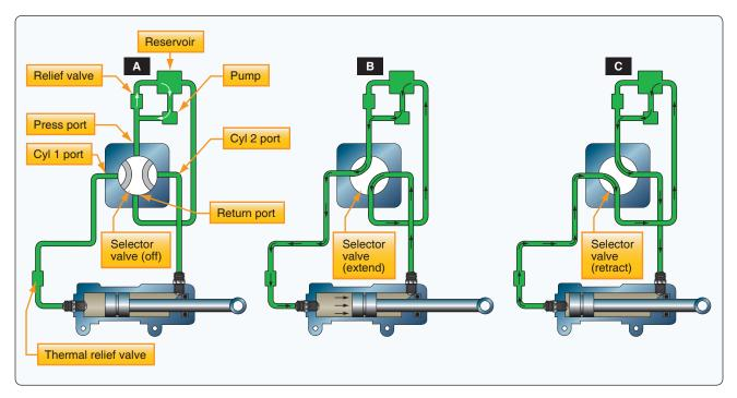
**Figure 12-33.** *Operation of a closed-center four-way selector valve, which controls an actuator.*
