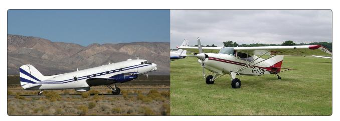
Figure 13-3. Tail wheel configuration landing gear on a DC-3 (left) and a STOL Maule MX-7-235 Super Rocket.
