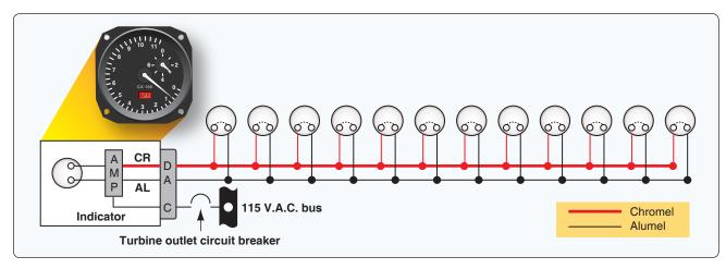
**Figure 10-74.** A typical exhaust gas temperature thermocouple system.
