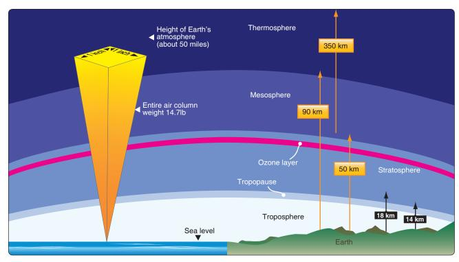
**Figure 16-34.** The weight exerted by a 1 square inch column of air stretching from sea level to the top of the atmosphere is what is measured when it is said that atmospheric pressure is equal to 14.7 pounds per square inch.
