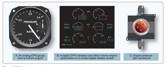
Figure 10-16. Engine pressure ratio gauges.
