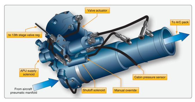
**Figure 16-64.** This pack valve drawing illustrates the complexity of the valve, which opens, closes, and modulates. It is manually actuated from the cockpit and automatically responds to supply and air cycle system parameter inputs.
