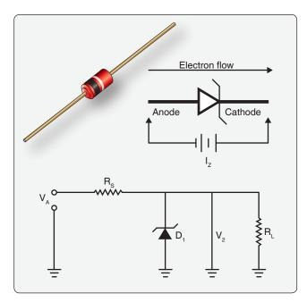
**Figure 11-25.** A zener diode, when reversed biased, will break down and allow a prescribed voltage to flow in the direction normally blocked by the diode.
