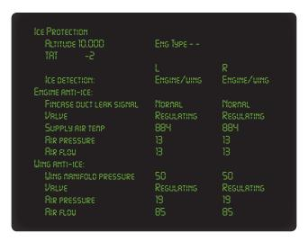
Figure 15-13. *Ice protection onboard computer maintenance page*.
