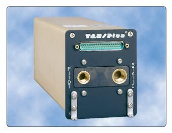
**Figure 10-28.** Teledyne's 90004 TAS/Plus air data computer (ADC) computes air data information from the pitot-static pneumatic system, aircraft temperature probe, and barometric correction device to help create a clear indication of flight conditions.
