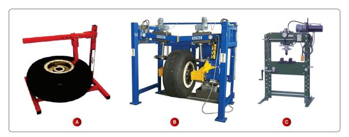
**Figure 13-63.** Tire beads must be broken from the wheel to remove the tire. A mechanical removal tool designed for breaking the bead is shown in (A); a hydraulic press designed with the capacity for large aircraft wheels is shown in (B); and an arbor press is shown in (C). All are tools available to the technician for this purpose.
