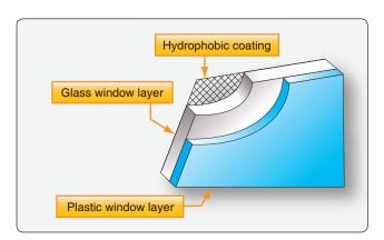
Figure 15-42. Hydrophobic coating on windshield.
