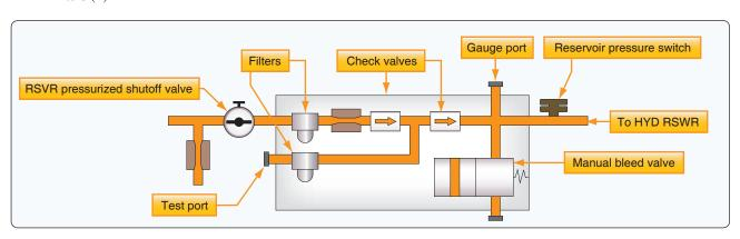
**Figure 12-12.** *Reservoir pressurization module.*
