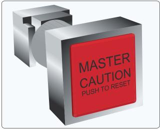
**Figure 10-129.** A master caution switch removed from the instrument panel.
