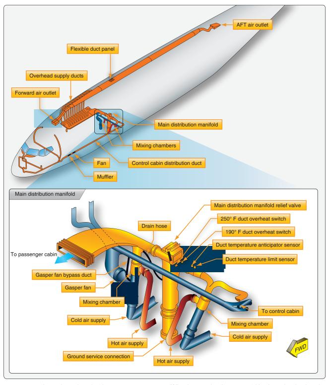
**Figure 16-60.** The conditioned air distribution system on a Boeing 737. The main distribution manifold is located under the cabin floor. Riser ducts run horizontally then vertcally from the manifold to supply ducts, which follow the curvature of the fuselage carrying conditioned air to be released in the cabin.
