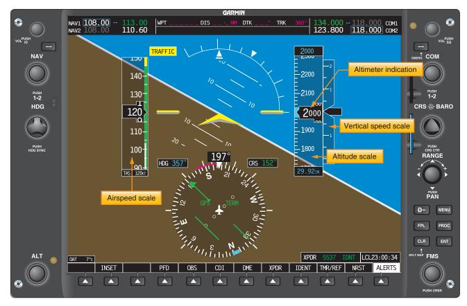
**Figure 10-34.** This primary flight display unit of a Garmin 1000 series glass cockpit instrumentation package for light aircraft indicates altitude using a vertical linear scale and a numerical counter. As the aircraft climbs or descends, the scale behind the black numerical altitude readout changes.
