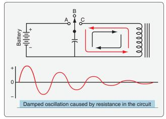
**Figure 11-58.** A tank circuit alternately charges opposite plates of a capacitor through a coil in a closed circuit. The oscillation is an alternating current that diminishes due to resistance in the circuit.
