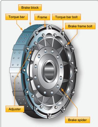
Figure 13-90. An expander tube brake assembly.
