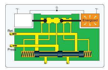
Figure 12-37. Servo control valve right solenoid energized.
