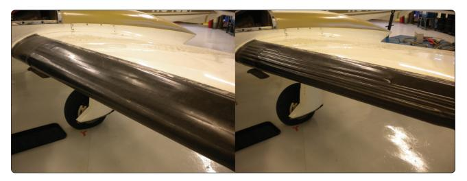
Figure 15-31. Deicing boots inflated (left) and deflated (right).
