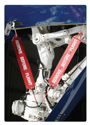
Figure 13-42. Gear pin ground lock devices.
