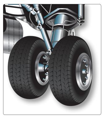
Figure 13-8. Dual main gear of a tricycle-type landing gear.
