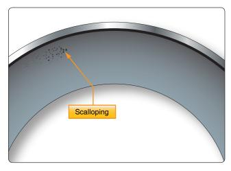
Figure 13-62. Improper loose torque on the axle nut can cause excessive end play leading to bearing race damage known as scalloping. Eventually, this leads to bearing failure.
