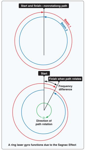
Figure 10-96. Light traveling in opposite directions around a nonrotating path arrives at the end of the loop at the same time (top). When the path rotates, light traveling with the rotation must travel farther to complete one loop. Light traveling against the rotation completes the loop sooner (bottom).
