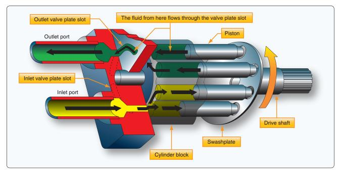
Figure 12-25. Axial inline piston pump.
