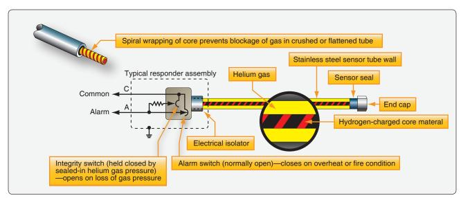
**Figure 17-7.** *Pneumatic pressure loop detector system.*
