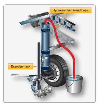
**Figure 13-26.** Air trapped in shock strut hydraulic fluid is bled by exercising the strut through its full range of motion while the end of an air-tight bleed hose is submerged in a container of hydraulic fluid.
