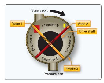
Figure 12-77. Schematic of vane-type air pump.
