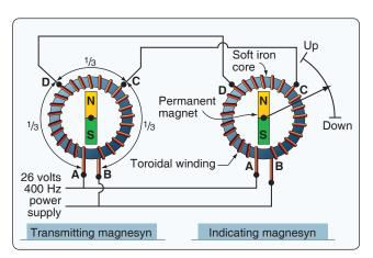
**Figure 10-49.** A magnasysn synchro remote-indicating system uses AC. It has permanent magnet rotors in the transmitter and indictor.
