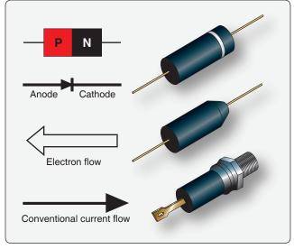
Figure 11-23. Symbols and drawings of semiconductor diodes.
