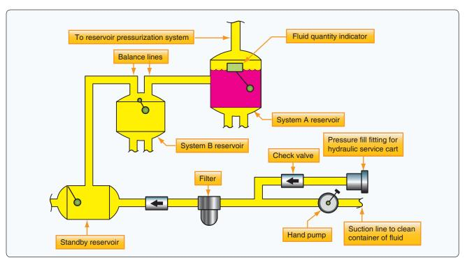
**Figure 12-14.** The hydraulic ground serive station on a Boeing 737 provides for hydraulic fluid servicing with a hand pump or via an external pressure fluid source. All three reservoirs are serviced from the same location.
