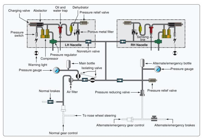
Figure 12-70. High-pressure pneumatic system.
