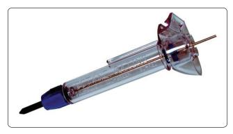
**Figure 14-93.** A sump drain tool used to open and collect fuel and contaminants from the fuel system sumps. Daily sump draining is part of the procedures needed to remove water from fuel that is to be delivered to the engine(s).
