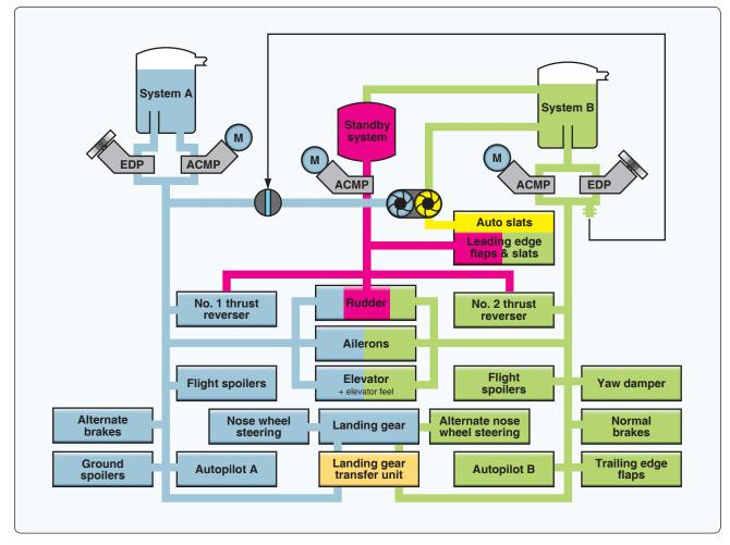
Figure 12-64. Boeing 737 hydraulic system (simplified).
