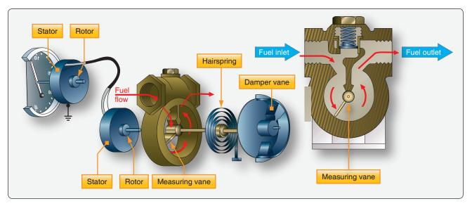
**Figure 14-77.** A vane-type fuel flow meter. Greater flow volume increases deflection of the vane against a calibrated spring. An autosyn transmitter replicates the vane shaft rotation on the cockpit indicator that is calibrated in gallons or pounds of fuel flow per hour.
