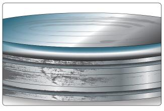
**Figure 13-72.** Bearing cups should be tight in the wheel boss and should never rotate. The outside of a bearing cup that was spinning while installed in the wheel is shown.
