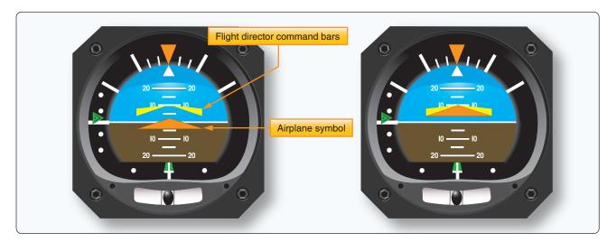
Figure 10-114. The fight director command bar signals the pilot how to steer the aircraft for a maneuver. By flying the aircraft so the triangular airplane symbol fits into the command bar, the pilot performs the maneuver calculated by the flight director. The instrument shown on the left is commanding a climb while the airplane is flying straight and level. The instrument on the right shows that the pilot has accomplished the maneuver.
