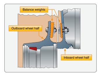
**Figure 13-77.** Two piece aircraft wheels are statically balanced when manufactured and may include weights attached to each wheel half that must stay with the wheel during its entire serviceable life.
