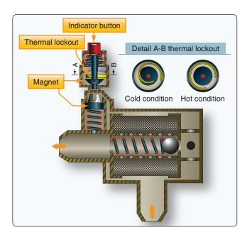
Figure 12-18. Filter bypass valve.
