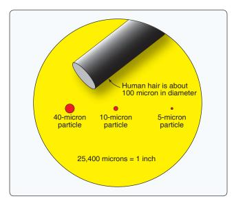
Figure 12-17. Size comparison in microns.
