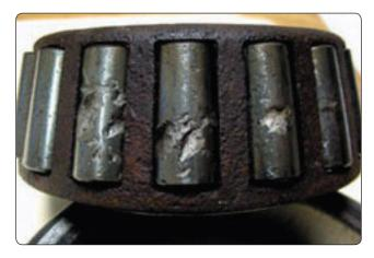
**Figure 13-65.** Spalling is a chipped away portion of the hardened surface of a bearing roller or race.
