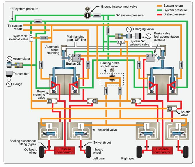
Figure 13-99. The power brake system on a Boeing 737.
