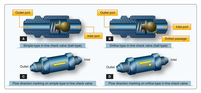
Figure 12-38. An in-line check valve and orifice type in-line check valve.
