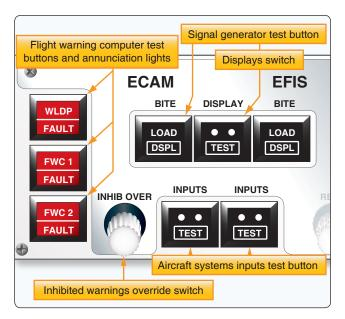
**Figure 10-123.** *An ECAM maintenance panel used for testing and annunciating faults in the ECAM system.*
