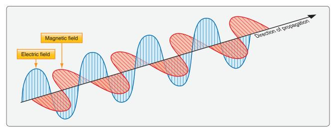
**Figure 11-77.** The electric field and the magnetic field of a radio wave are perpendicular to each other and to the direction of propagation of the wave.
