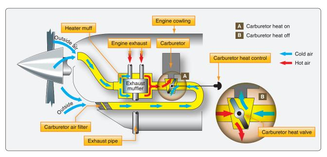
**Figure 14-6.** To combat carburetor icing, air preheated by the exhaust manifold is directed into the carburetor via a push/pull control in the cockpit. The control changes the position of the air diverter butterfly in the carburetor heat valve box.
