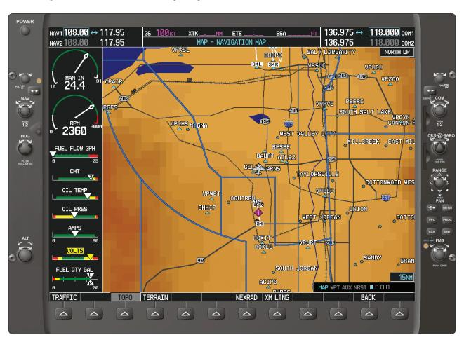
**Figure 10-14.** Oil pressure indication with other engine-related parameters shown in a column on the left side of this digital cockpit display panel.
