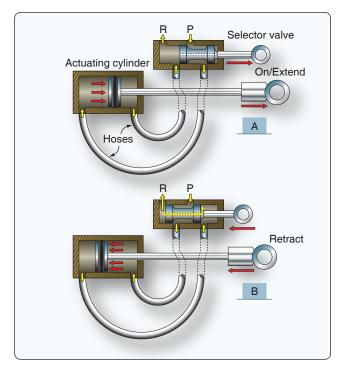
Figure 12-53. Linear actuator operation.
