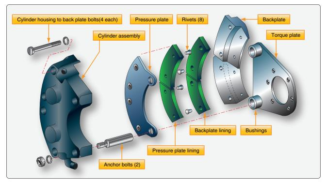
Figure 13-123. A Cleveland brake disassembles once the four bolts holding the cylinder to the backplate are removed while the aircraft wheel remains in place. The pressure plate slides off the anchor bolts and linings can be replaced by riveting on the pressure plate and back plate.
