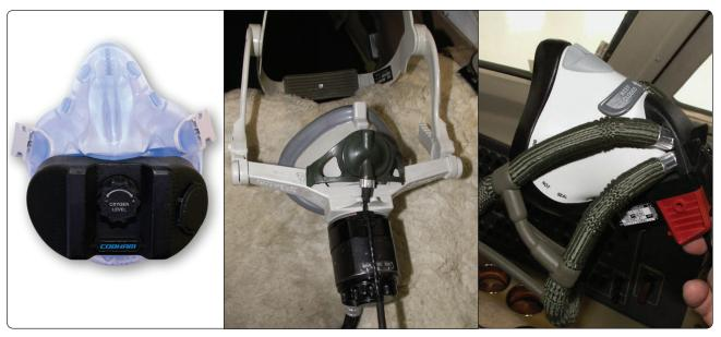
Figure 16-22. A mask-mounted version of a miniature diluter-demand regulator designed for use in general aviation (left), a mechanical quick-donning diluter-demand mask with the regulator on the mask (center), and an inflatable quick-donning mask (right). Squeezing the red grips directs oxygen into the hollow straps.
