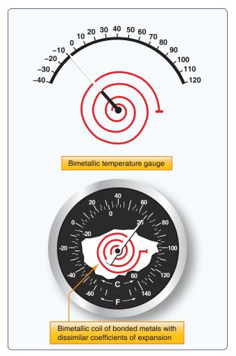
Figure 10-66. A bimetallic temperature gauge works because of the dissimilar coefficients of expansion of two metals bonded together. When bent into a coil, cooling or heating causes the dissimilar metal coil to tighten, or unwind, moving the pointer across the temperature scale on the instrument dial face.
