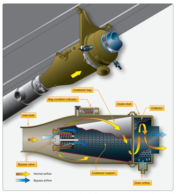
**Figure 16-68.** A water separator coalesces and removes water by swirling the air/water mixture from ACM expansion turbine. Centrifugal force sends the water to the walls of the collector where it drains from the unit.
