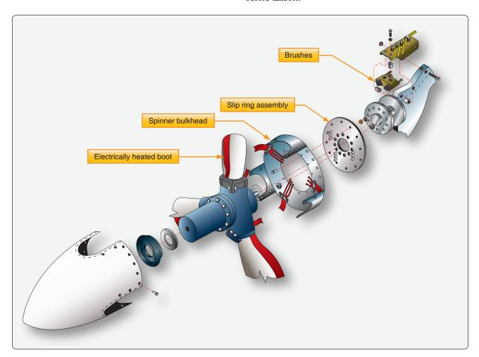
Figure 15-35. Electro thermal propeller deice system components.
