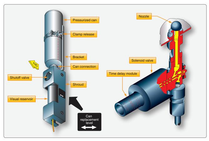
Figure 15-41. Cockpit rain repellant canister and reservoir.
