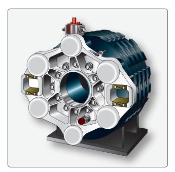
**Figure 13-89.** *A carbon brake for a Boeing 737.*
