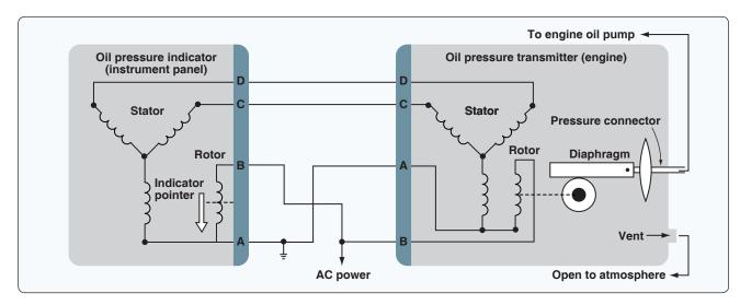
**Figure 10-51.** Remote pressure sensing indicators change linear motion to rotary motion in the sensing mechanism part of the synchro transmitter.
