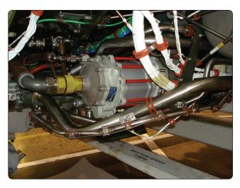
Figure 12-21. Engine-driven pump.
