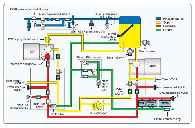
**Figure 12-67.** Right hydraulic system of a Boeing 777. A left system is similar.
