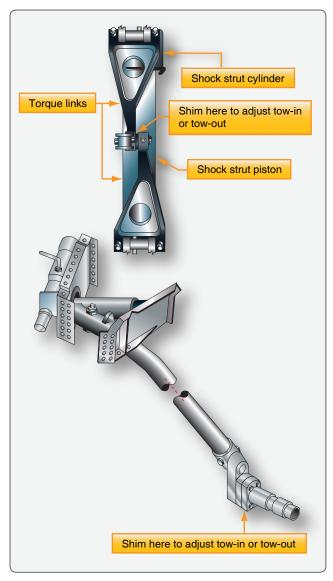
Figure 13-31. Tow-in and tow-out adjustments on small aircraft with spring steel landing gear are made with shims behind the axle assembly. On shock strut aircraft, the shims are placed where the torque links couple.
